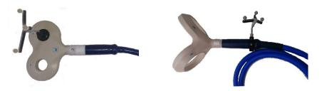
Figure 2-1. Figure 8 (left) and Double-cone (right) TMS coils. The circular parts of the coil contain windings that generate focus the magnetic field. The magnetic field generated by the figure 8 coil reaches maximum intensity approximately 2cm below the centre point of the coil, where the two circular windings meet. The point of maximum magnetic intensity with the double-cone coil occurs between the two coil windings, approximately 5cm from the handle.
