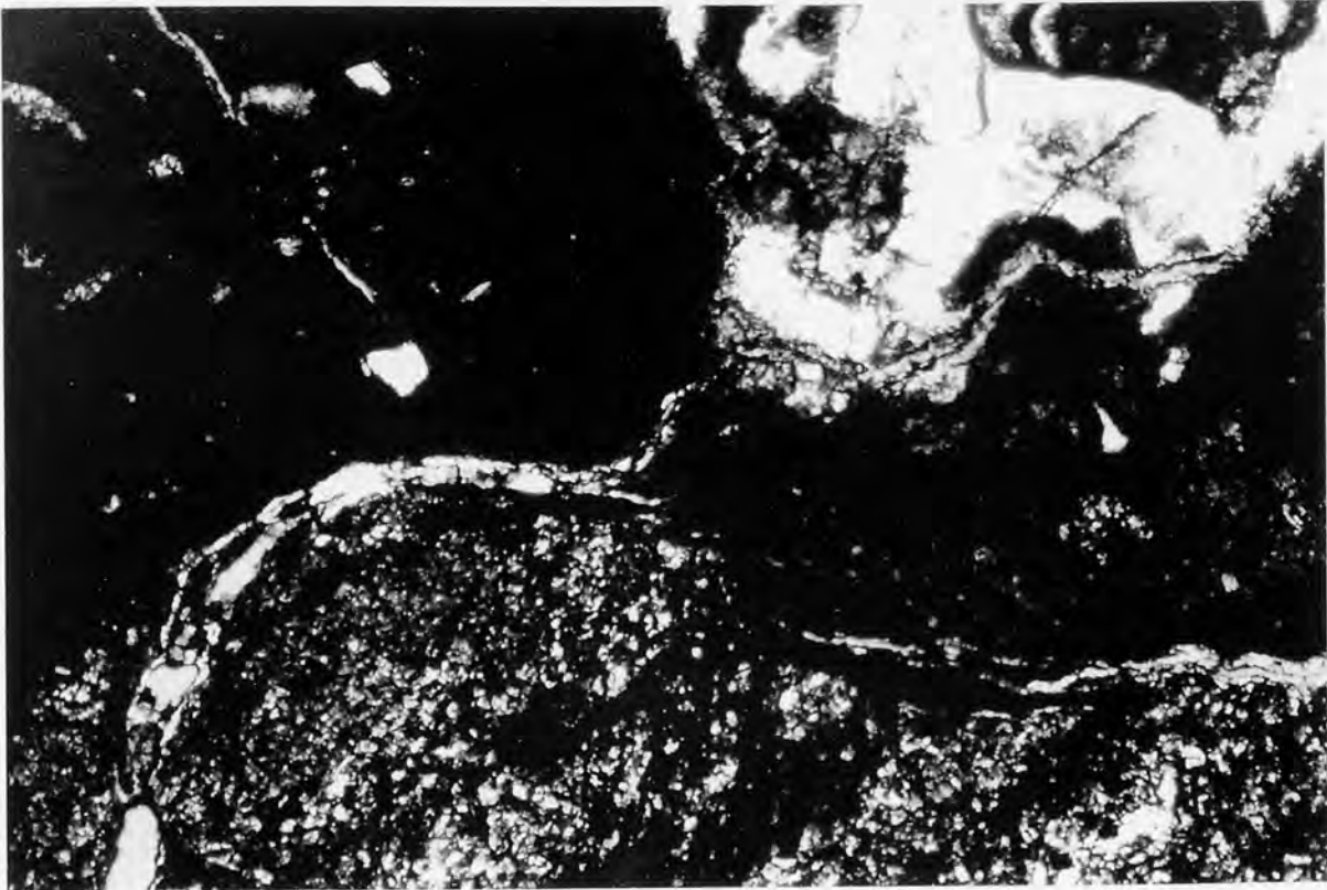
Plate 4.2 Extensive ASR microcracking containing some ASR gel, developed within the siltstone aggregate and continuing out into the surrounding cement paste. Dry Rigg siltstone mix, 3 \text{ kg/m}^3 \text{ Na}_2\text{O}_e (Sample No. DR23.0A, immersed in salt solution plane polarised light, X40 Mag).
