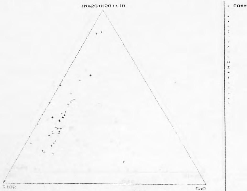
FIGURE 7.8: Ternary compositional diagram, \text{SiO}_2 : \text{Na}_2\text{O} + \text{K}_2\text{O} : \text{CaO} of ASR gel from within coarse aggregate particles, (CA). Concrete Name: Dry Rigg siltstone 7 \text{ kg/m}^3 \text{ Na}_2\text{O}_e immersed in salt solution for 15 months.
