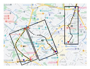
Fig. 1: Three central Birmingham areas monitored before and during the 2022 Commonwealth Games: sensors 1 and 2 measure inflow traffic; the unlabeled sensor captures outflow traffic.
