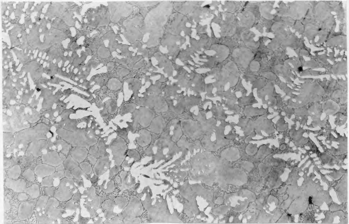
Figure 5.60. Optical micrograph of ACuZinc5 tested at 100 MPa and 160°C, at low magnification. (100×)
