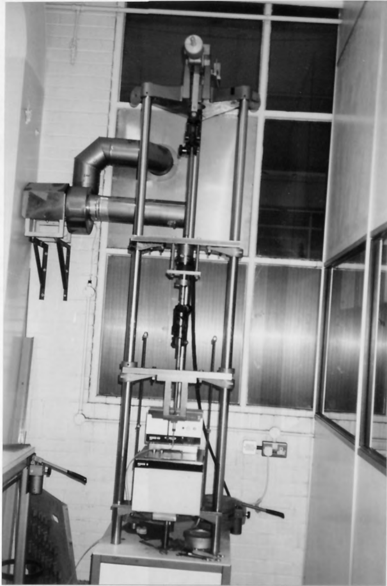
Figure 3.1. Designed compressive creep machine with oil-bath.
