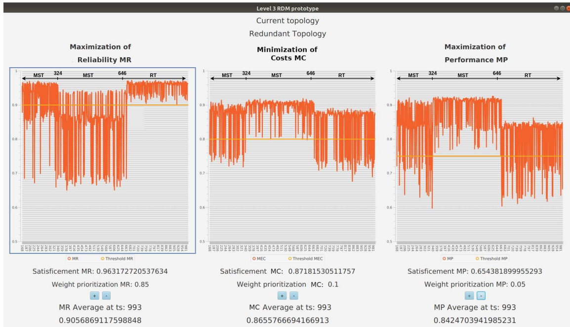
Figure 6.9: GUI showing the system’s historical behavior. At time slice 646, the user set a higher priority to the MR NFR (left chart).
