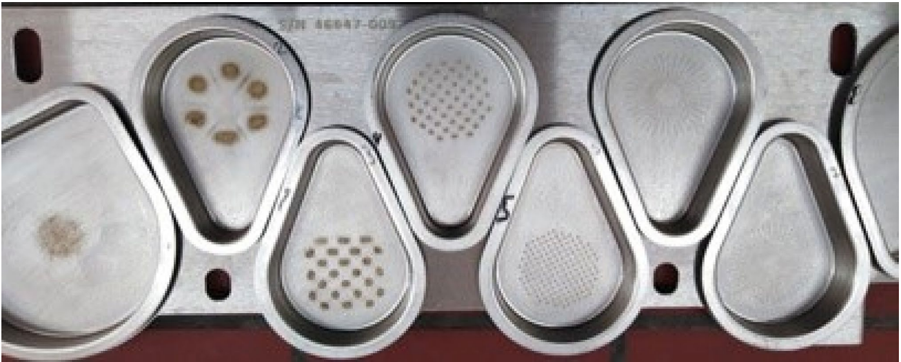
Fig. 5 Deposition of the chitosan date nanoparticles onto the NGI apparatus highlights the brown powder from trays 1 to 7 (labeled from left to right)
