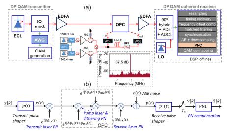
Figure 1. (a) Experimental setup showing the dual-polarisation 28-Gbaud M-QAM transmitter, the dual-pump OPC device, the coherent receiver, and the offline DSP. Inset: RF spectrum of coherently received conjugated continuous-wave signal after the OPC with optimised pump dithering. (b) Conceptual model of the various sources of noise in the OPC transceiver.
