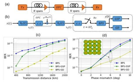
Figure 3. (a) Schematic of mid-link OPC transmission system. (b) Baseband channel model. (c) BER after BPS, BPS-GSP and BPS-GD PN compensation versus transmission distance in the link at a pump-phase mismatch of  $\delta\theta = 6^{\circ}$ . (d) BER versus pump phase mismatch after 1200-km transmission. The inset shows the signal constellation diagrams for  $\delta\theta = 6^{\circ}$ .
