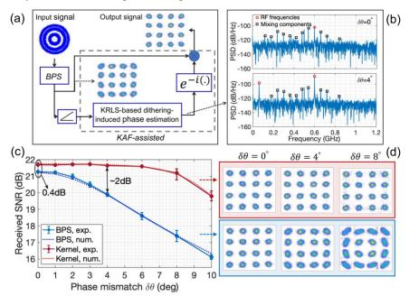
Figure 2. (a) Block diagram of the KRLS-based PN compensation scheme. (b) Spectral representation of the estimated PN after the KAF unit for 16-QAM. (c) Received SNR versus pump-phase mismatch  $\delta\theta$  for 16-QAM
