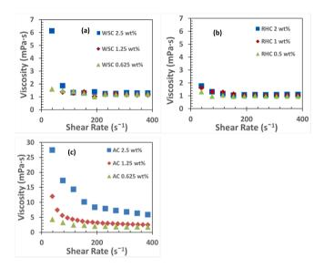
Fig. 7. The effect of shear rates and nanoparticle concentrations on the viscosity of nanofluids: a) WSC, b) RHC and c) AC. The viscosity measurements were carried out at pH6 and a temperature of 22  $^{\circ}$ C.
