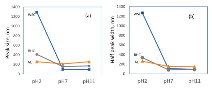
Fig. 5. The centre of the particle size distribution peak (a) and half peak width (b) at selected pH values determined by Dynamic Light Scattering (DLS).
