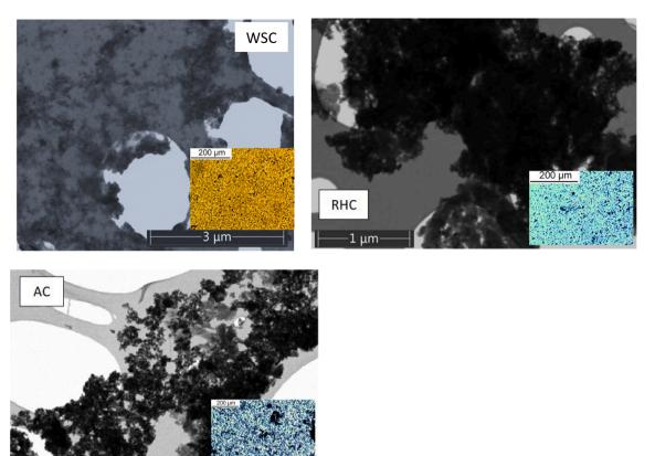
Fig. 3. Electronic and optical microscopic images of the nanofluids prepared from WHS, RHC or AC, respectively. The optical microscopic images are the inset.
