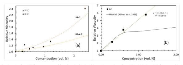
Fig. 8. Relative viscosity of nanofluids versus nanoparticle volumetric fraction: (a) experimental data of the WSC and RHC nanofluids compared to the calculated values using the modified Chen equation (the dotted lines) and (b) the AC nanofluids (the solid square with the regression line) compared to that of carbon nanotube nanofluids (the solid black line). The viscosity was measured at pH6, 100 rpm and 22°C.
