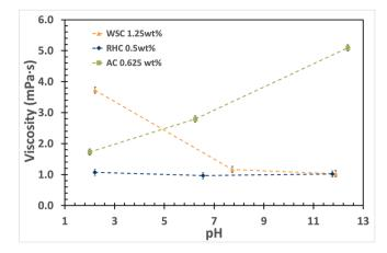
Fig. 6. The effect of pH values of the nanofluids on their viscosities. The viscosity was measured at 100 rpm and 22  $^\circ\text{C}.$
