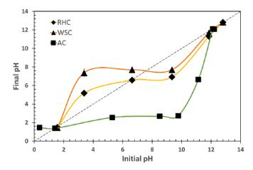
Fig. 2. The final pH value versus corresponding initial pH values for aqueous solutions containing RHC, WHS or AC. The dotted line represents y = x for finding an accurate PZC<sub>pH</sub> value.
