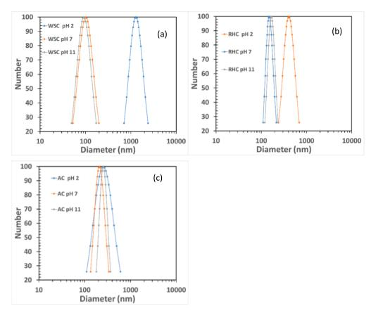
Fig. 4. Effect of pH values on the normalised particle number size distribution of a) WSC, b) RHC and c) AC determined by Dynamic Light Scattering (DLS).
