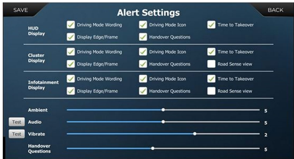
Fig. 6 The customisation matrix displayed at the end of each trial on the vehicle’s infotainment display
