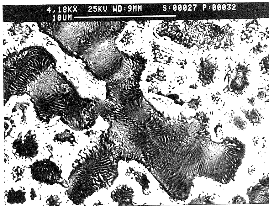
Figure 93. SEM.As-cast structure of ZA27K, showing the decomposition of \alpha' particles.
