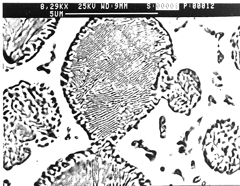
Figure 78. SEM.As-cast structure of ZA8K, showing b decomposed into well-formed lamellae and a mixture of phases.
