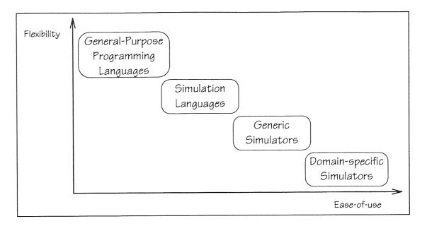
Figure 6-1 Trade-off between Ease-of-use and Flexibility in Approaches to Constructing Simulation Models
