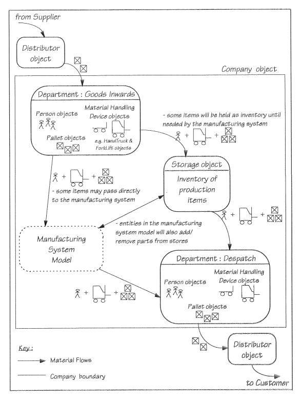
Figure 9-3 An Object Model of a Stores Function
