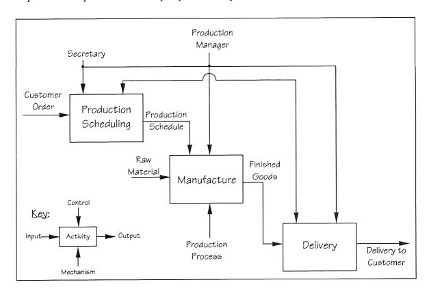
Figure 5-2 IDEF0 Model of a Make-to-Order Process (adapted from Plaia & Carrie, 1995)
