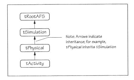
Figure 10-1 The Core Simulator Class Hierarchy in AFS
