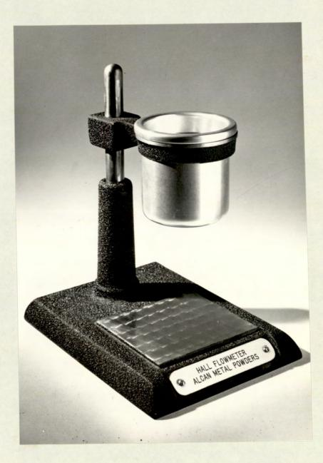
For commercially available powders, apparent density is generally in the range 20-50% of the theoretical density of the solid material. Its value is controlled by other powder properties, such as:
