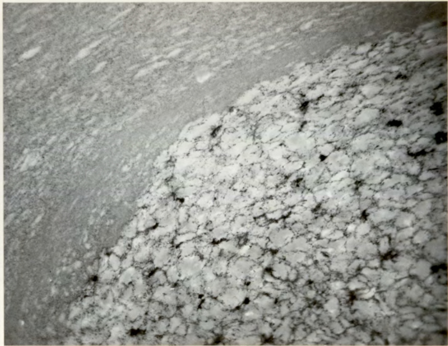
12. Screw cross channel section showing forward fusion mechanism with Solvic VP 17/10 dryblend.
