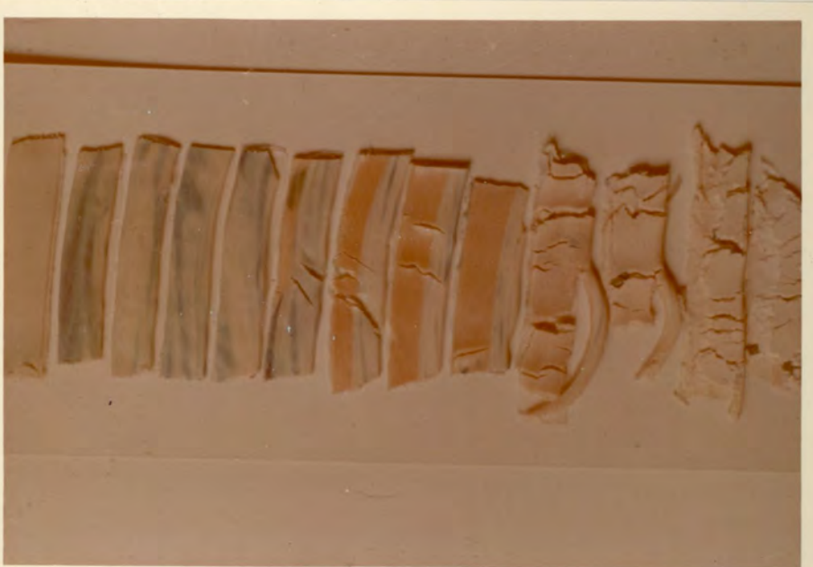
9. Material removed from screw channel - rear fusion mechanism with PVC dryblend containing coloured marker granules.
