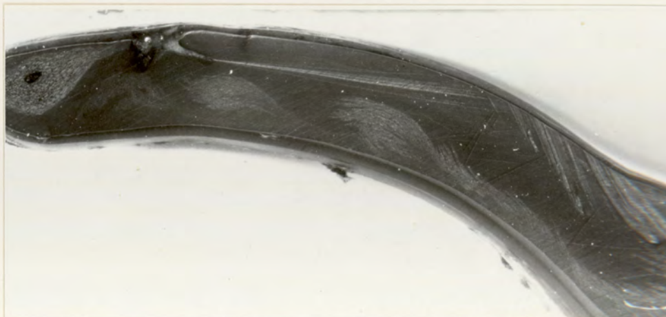
5. Screw channel cross section showing entrapped air and patches of unfused PVC.
