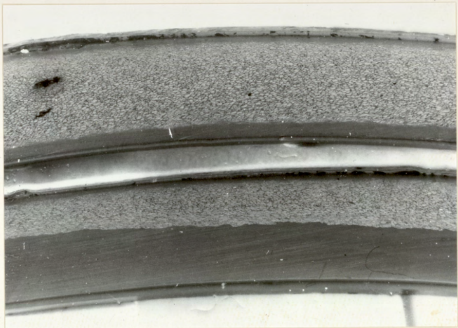
6 Screw down channel section showing rear fusion mechanism - intermediate stage.
