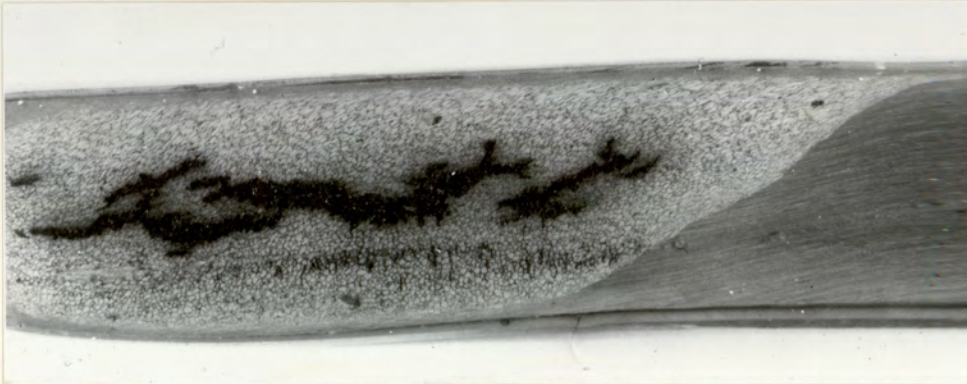
3. Screw cross channel section showing rear fusion mechanism - intermediate stage.
