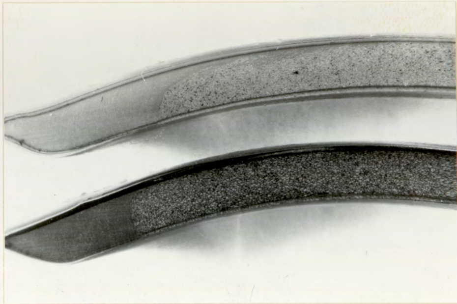
10. Screw cross channel section showing forward fusion mechanism with Solvic VP 17/10 (above) and PVC dryblend containing 1 phr Wax E. (below)
