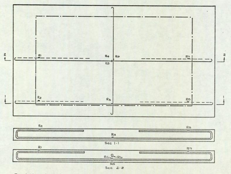
Fig. 9.14. Location of strain gauges on reinforcement bars. test Mz.
