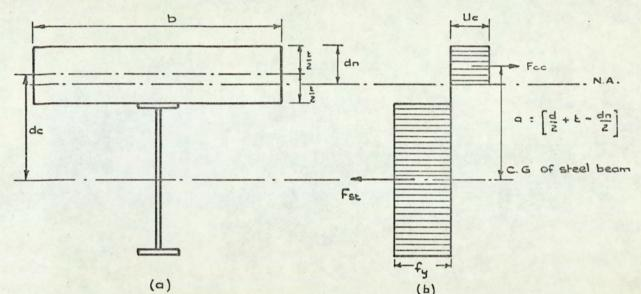
(a) Fig. 5.1. Section and stress diagram for a composite beam with the neutral axis within the concrete slab, Ignoring slab reinforcement.
