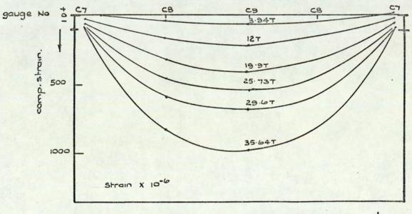
Fig. 10. 4. Distribution of strain along the transverse  $\xi$  of the slab upper surface. Test M<sub>1</sub>.
