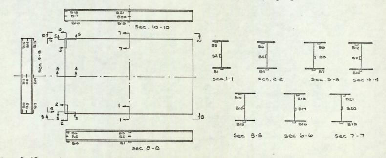
Fig. 9. 12. Location of strain gauges on the steel frame. Test. MI.
