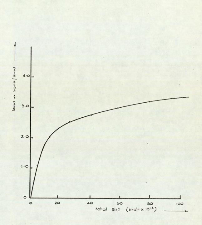
Fig 9.6. Load v. slip characteristics of  $\frac{1}{2}$  in. diameter 2 in. high mid steel stud shear connector,
