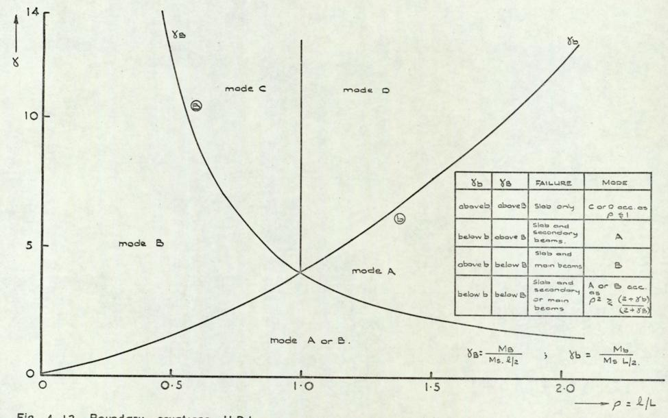
Fig. 4.12. Boundary equations. U.D.L. no composite action. slab continous in four directions.
