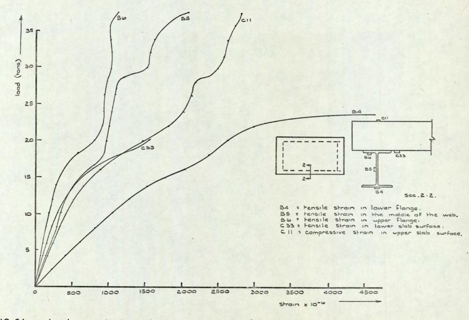
Fig. 10. 24. Load against strain for main composite beam at mid-span. Test M2.
