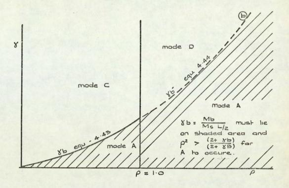
Fig. 4.10. Comparison of collapse modes for internal bay. U.D.L. for mode A to occur.
