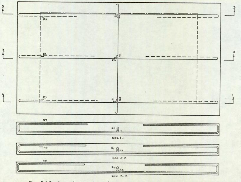
Fig. 9.10. Location of strain gauges on reinforcement bars test Mi.
