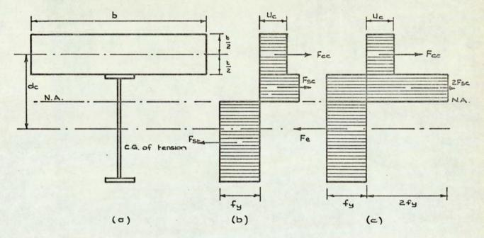
Fig. 5.2. Section and stress diagram for a composite beam with the neutral axis within the steel beam. Ignoring slab reinforcement.
