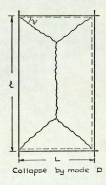
Fig 4.4. External bay of multi-bay continious frame. Basic modes of collapse for U.D.L.
