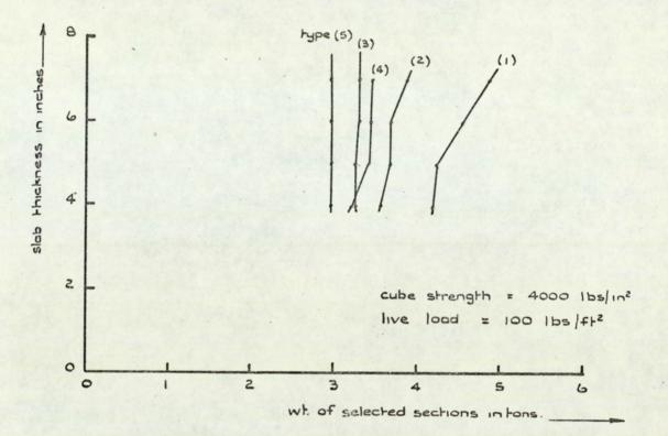
Fig. 7.14. Weight of the selected supporting beams of frame I for the five types of assumptions on degree of composite action, for different slab thicknesses.
