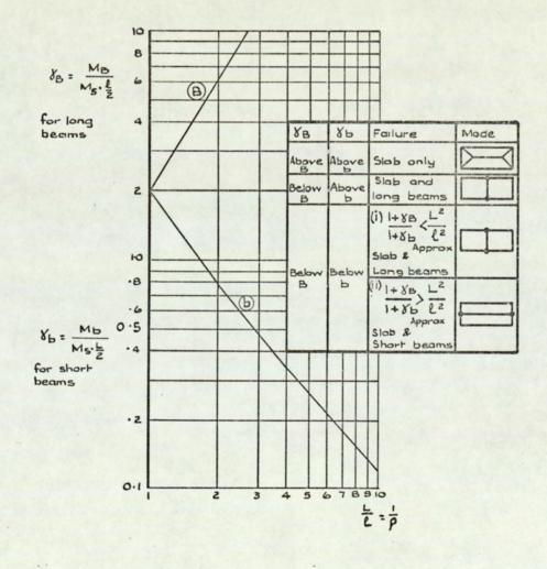
Fig. 3.4. Boundary equations for a simply supported rectangular slab. U.D.L.
