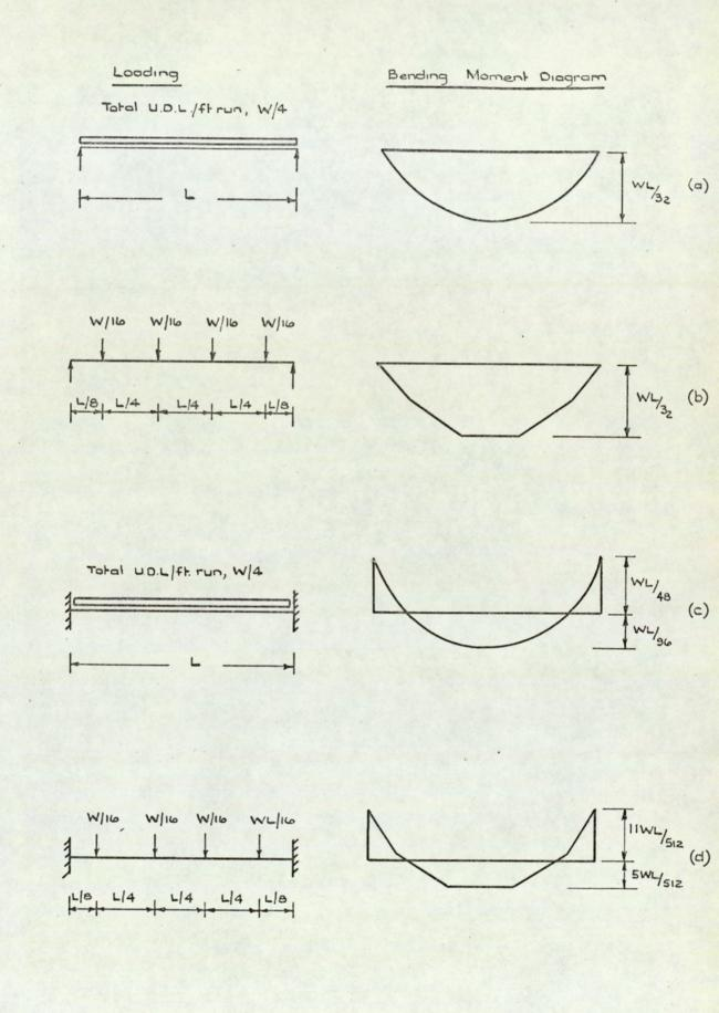
Fig. 9.7. Limits of end conditions of slab and main edge beams. Tests  $M_1$  and  $M_2$ .
