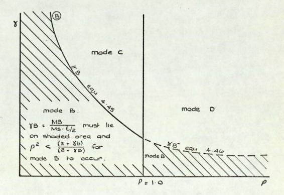
Fig. 4.11. Comparison of collapse modes for internal bay. U.D.L. for mode B to occur.
