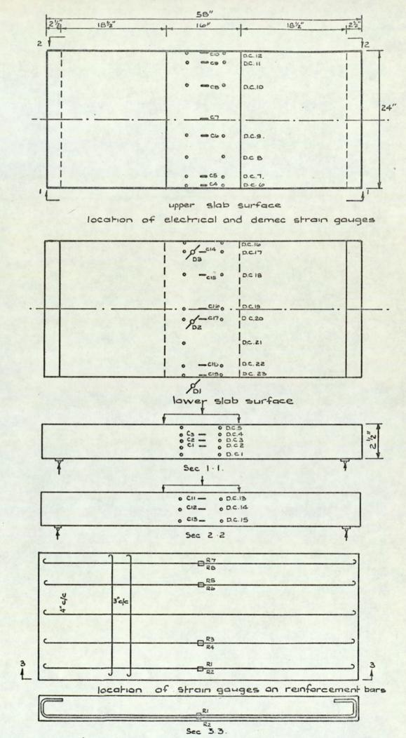
Fig. 9. 21. Dimensions and gauging of slab strips Si & Sz.
