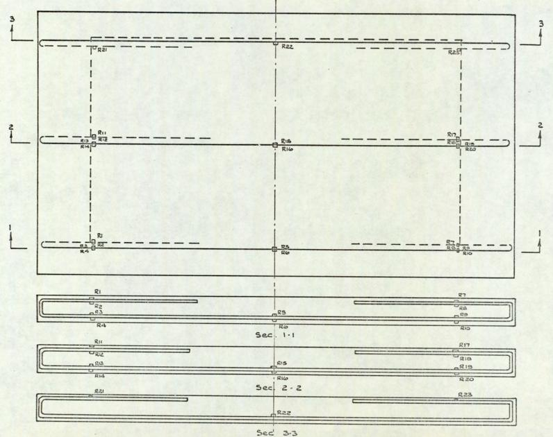
Fig. 9, 18. Location of strain aquaes on reinforcement bars test Ma
