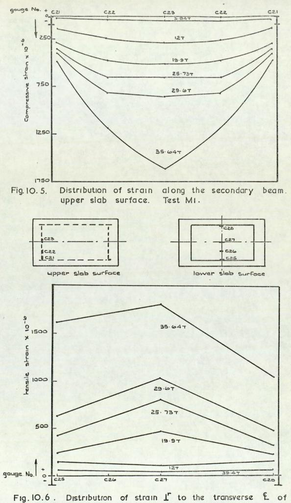
the lower slab surface. Test MI.
