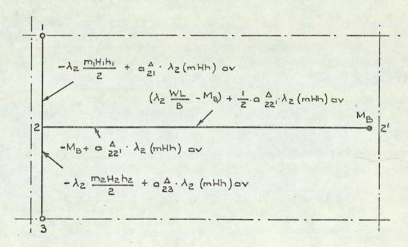
Fig. 8.8.(b) Bending moments at ultimate combined load - Zone 2(i). 8.7.2(b) ZONE II (ii)
