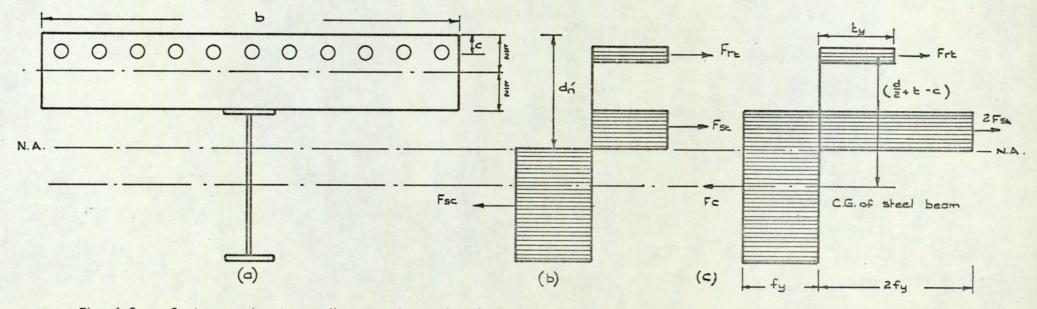
Fig 6.2 Section and stress diagram for a hogging composite beam with the neutral axis within the steel beam.
