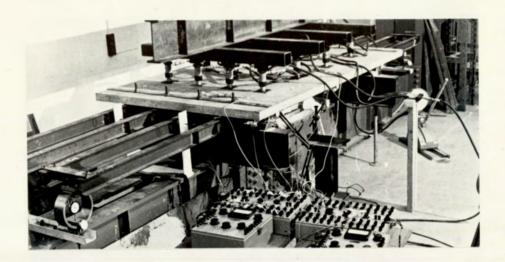
Plate 8. Details of lever arm system.
