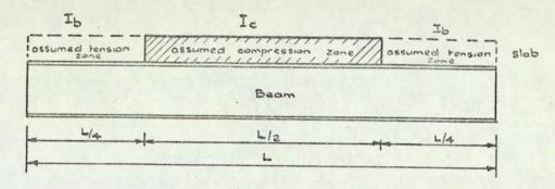
Fig. 8.11. Assumed effect of composite action on the beam span.
