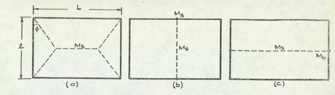
Fig. 3.3. Collapse of a simply supported rectangular slab under a U.D.L.
