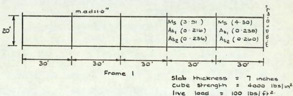
Fig. 7.6. The complete design of frame I for each of the five types of assumptions on degree of composite action.
