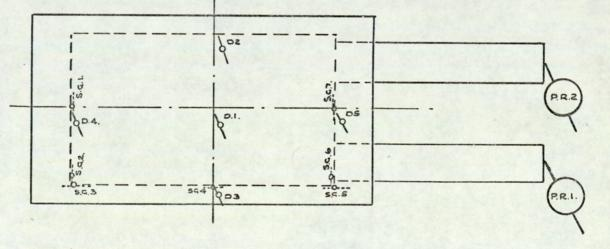
Fig. 9.16. Location of deflection, slip and proving ring gauges. Test M2.
