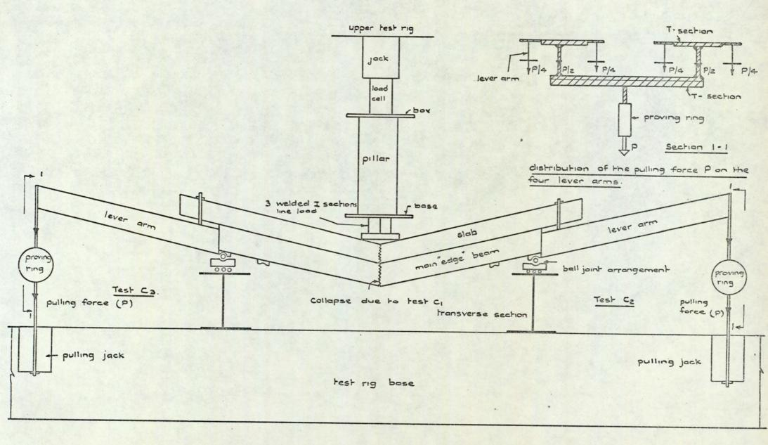
Fig. 9.8. Control tests C2 and C3 set up.
