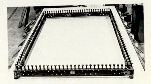
Plate 3. Stud shear connectors welded on top of the steel frame of the models.
