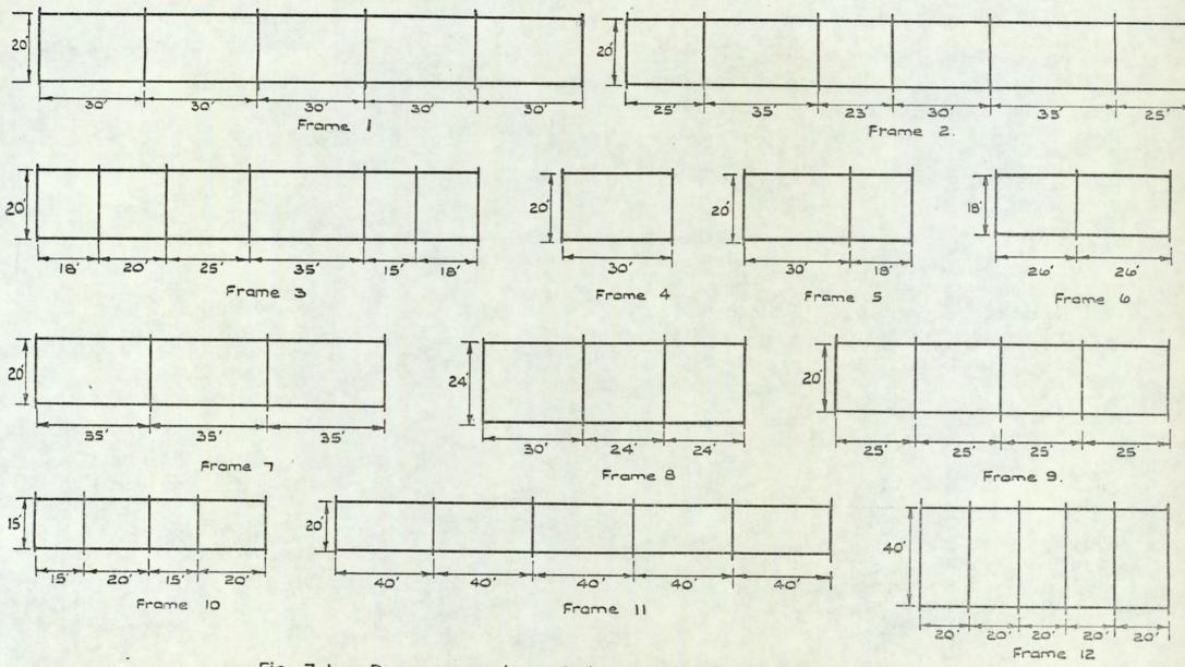
Fig. 7.1. Design examples of beam and slab floor systems.
