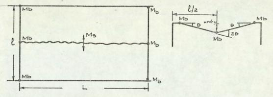
Collapse load by mode A (secondary beams at supports are rigidly jointed)
