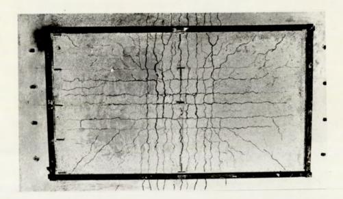
Plate 16. Pattern of cracks at lower slab surface of model Mi after test.
