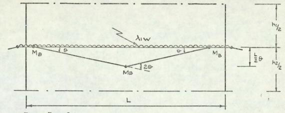
a. Zone I . Collapse mechanism under vertical load alone.
