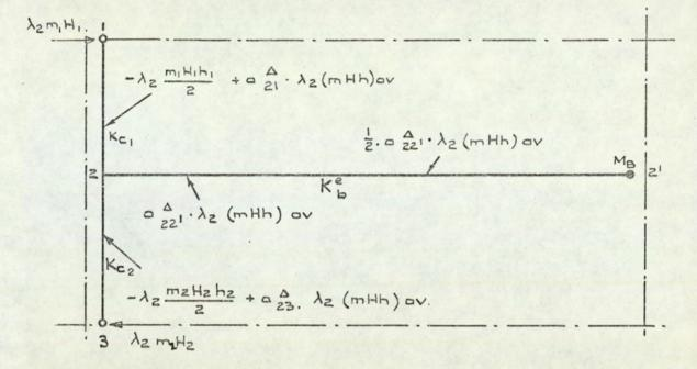
Fig 8.8.(a). Bending moments due to wind load alone - Zone 2.(i).
