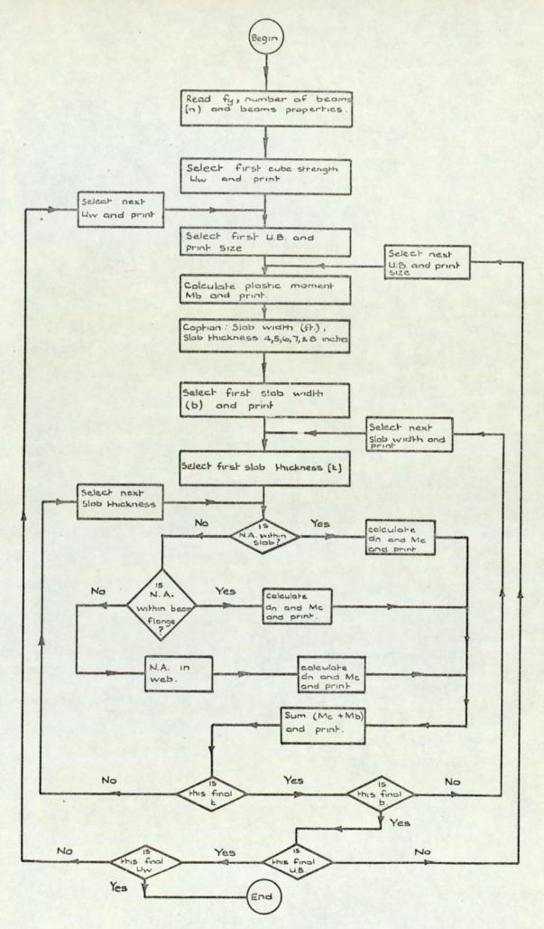
Fig. 5.7. Flow diagram for computer program to calculate  $M_b$ ,  $M_c$ ,  $d_n$ , and  $(M_c + M_b)$ .
