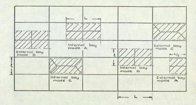
Fig. 4.1. Multi - bay continious beam and slab floor system.
