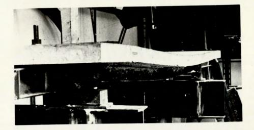
Plate 15. Final deflected shape of model M1 after test.
