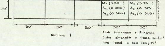
Fig. 7.5. The complete design of frame I for each of the five types of assumptions on degree of composite action.
