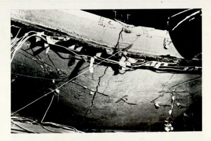
Plate 20. Formation of plastic composite hinges at mid-span of model M<sub>3</sub> after control test C<sub>1</sub>.
