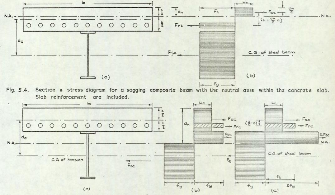
Fig. 5.5. Section a stress diagram for a sagging composite beam with the neutral axis within the steel beam Slab reinforcement are included.
