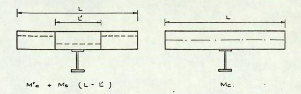
Fig. 5.3. Change in position of neutral axis by assuming the full effective width
