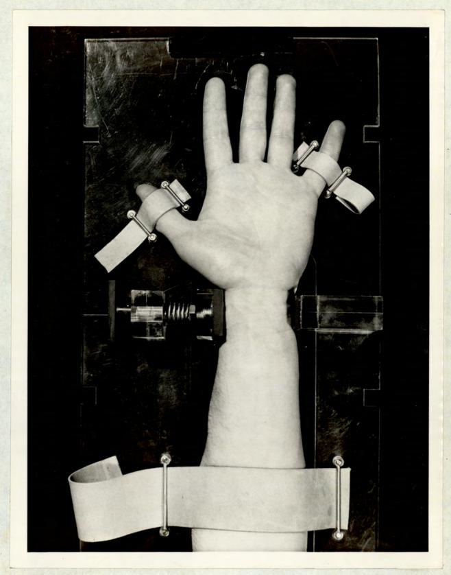
Fig. 3.11. Photograph showing a subject's arm fixed in the perspex frame.
