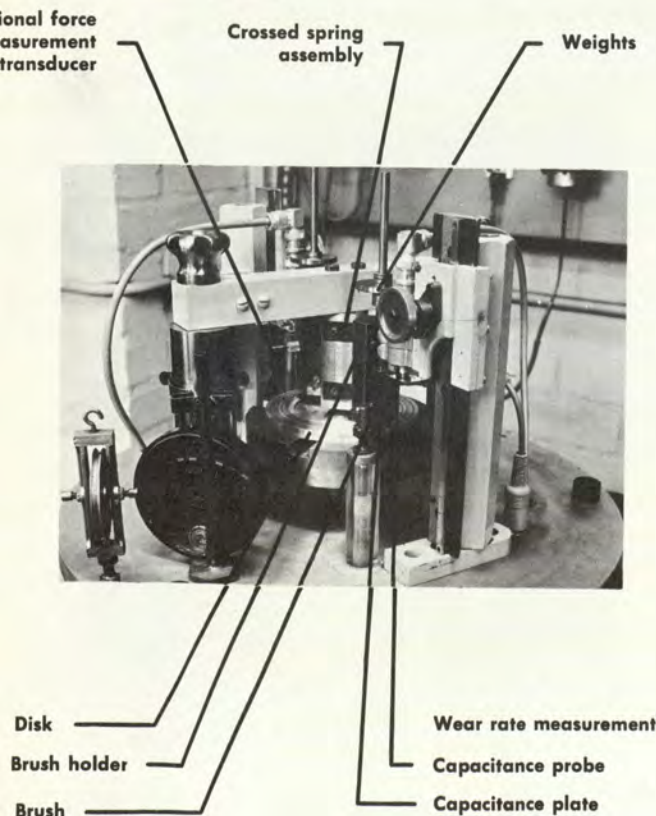
Fig. 1—Photograph of wear test rig showing disk, brushes and measurement transducers.
