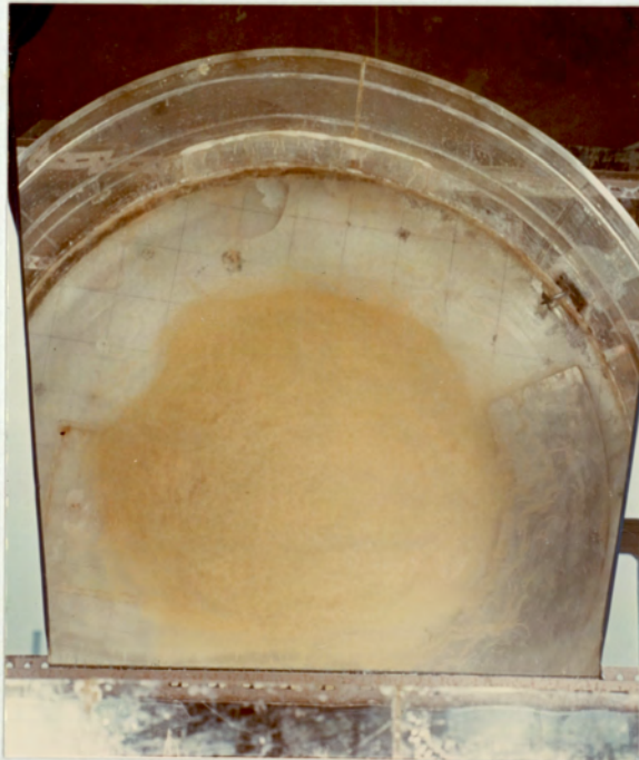
FIGURE 63 DISTRIBUTION OF PULP ON THE BASE OF THE TANK AT A SHAFT ANGLE OF A) 5^{\circ} B) 10^{\circ}
