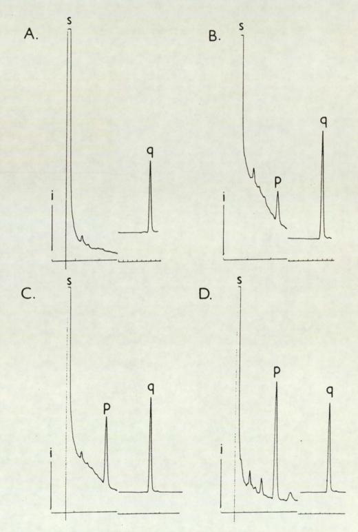
lonisation amplifier was set at 8 (0-3min) and 320 (3-12min). Abbrev: i, injection of sample; s, solvent front; p, propyl-Nmethylcarbamate; q, quinoline.
