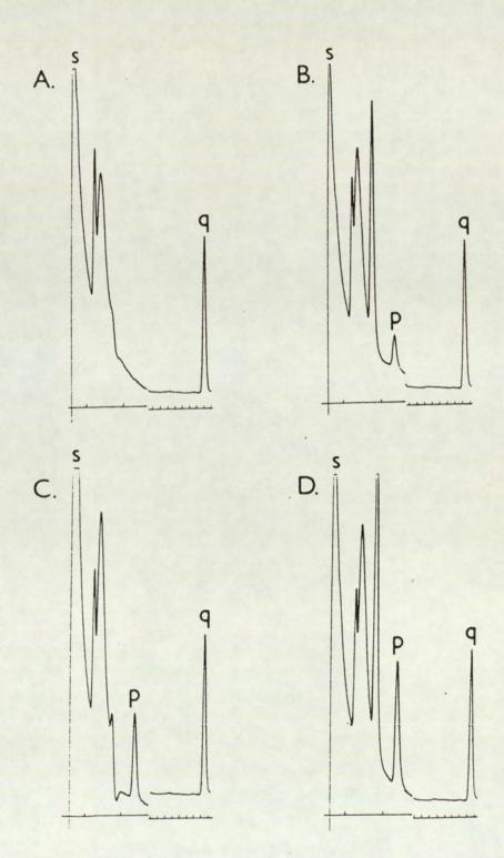
Ionisation amplifier was set at 8 (0-3min) or 160 (3-12min). Abbrev: s, solvent front; p, propyl-N-methylcarbamate; q, quinoline. Gas-liquid chromatograms of derivatised samples of mouse hepatocytes containing SEG (A, control; B,  $20\mu$ M; C,  $60\mu$ M; D,  $100\mu$ M).
