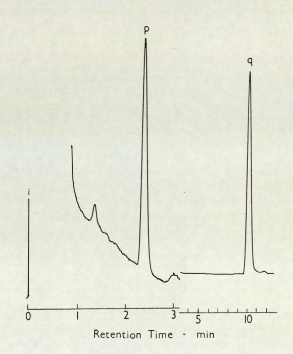
Ionisation amplifier was set at 8 (0-3min) or 320 (3-12min). Abbrev: i, injection of sample; p, propyl-N-methylcarbamate; q, quinoline. Figure 13
