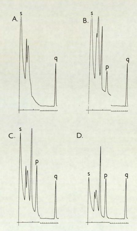
Ionisation amplifier was set at 8 (0-3min) and 160 (3-12min) except for D where it was set at 16 (0-3min) and 160 (3-12min). Abbrev: s, solvent front; p, propyl-N-ethylcarbamate; q, quinoline. Figure 15
