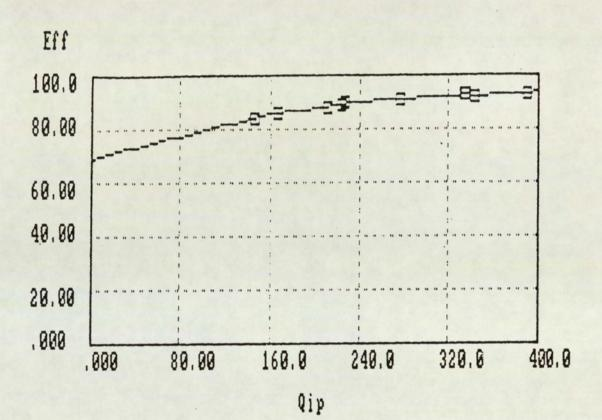
Calibration quench curve of counting efficiency (Eff).
