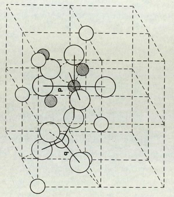
FIGURE 1.2 Spinel Structure (after Gorter, 1954)
