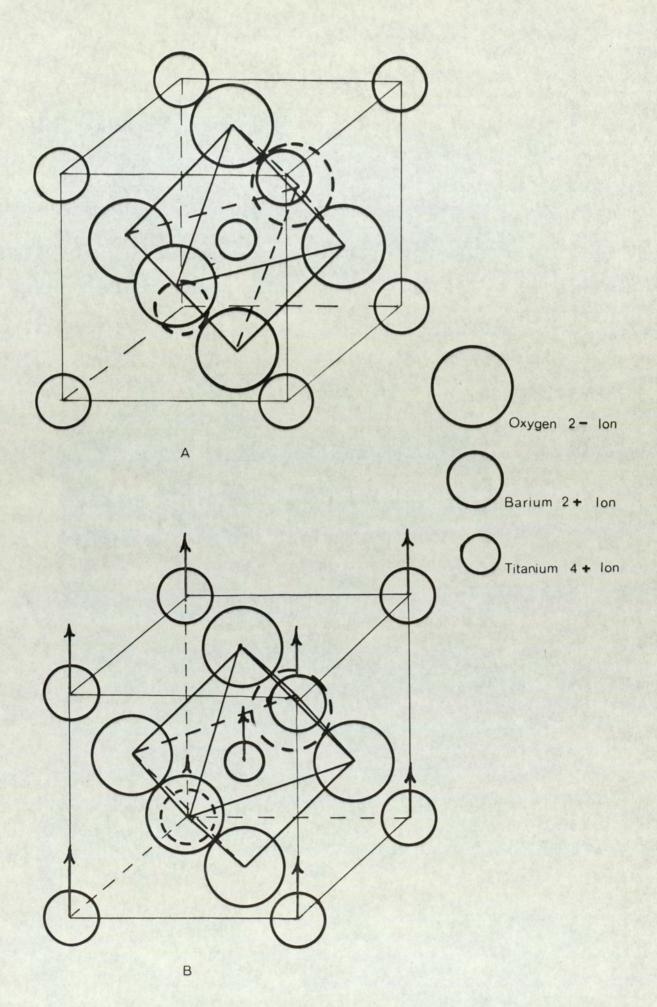
Figure 1.1 The Structure of Barium Titanate
