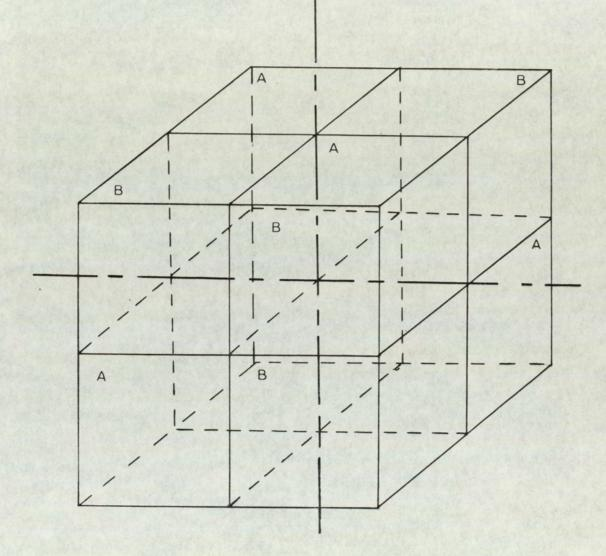
FIGURE 2.10 A unit cell of Spinel
