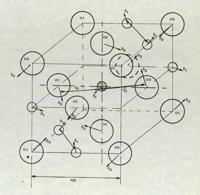
FIGURE 2.9 Section B of the Spinel structure
