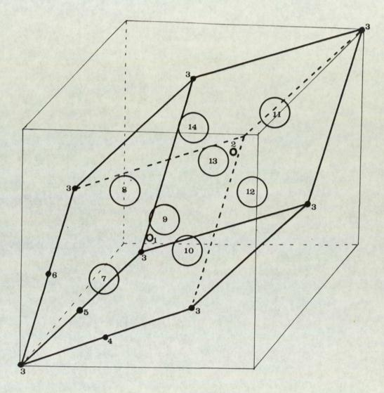
FIGURE 5.1 The Primitive Unit Cell of Spinel
