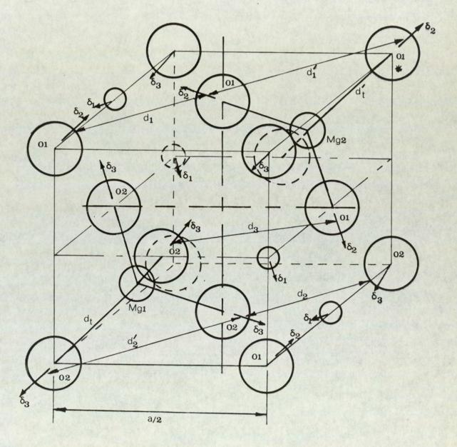
FIGURE 2.8 Section A of the Spinel structure
