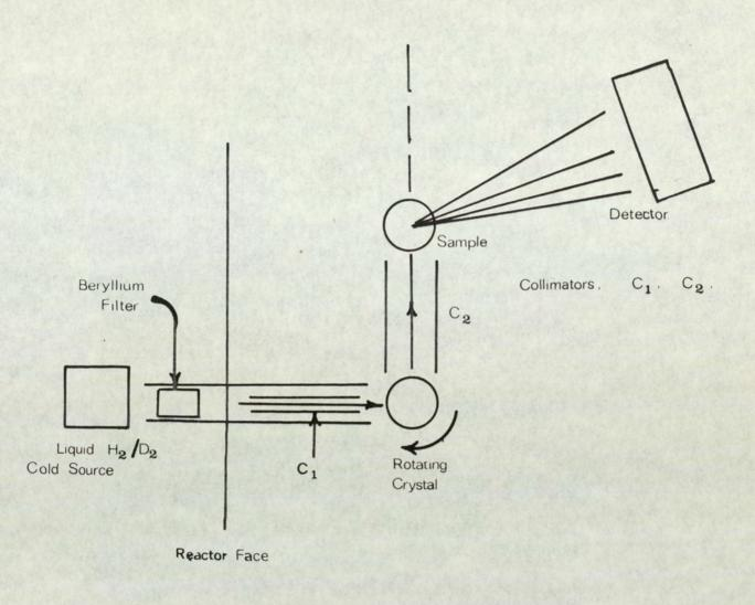
Fig 4. 1. Schematic View of R. X. S.
