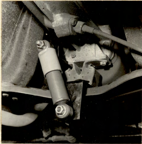
FIG. 4.3 INSTALLATION OF HYDRAULIC DAMPER, IN PARALLEL WITH THE REAR ENGINE/TRANSMISSION MOUNT.
