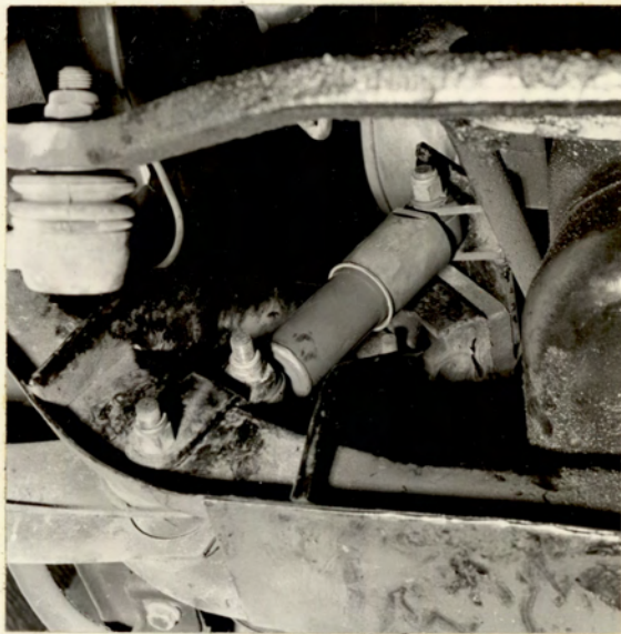
FIG. 4.4 INSTALLATION OF FRONT NEAR SIDE HYDRAULIC ENGINE/TRANSMISSION DAMPER.
