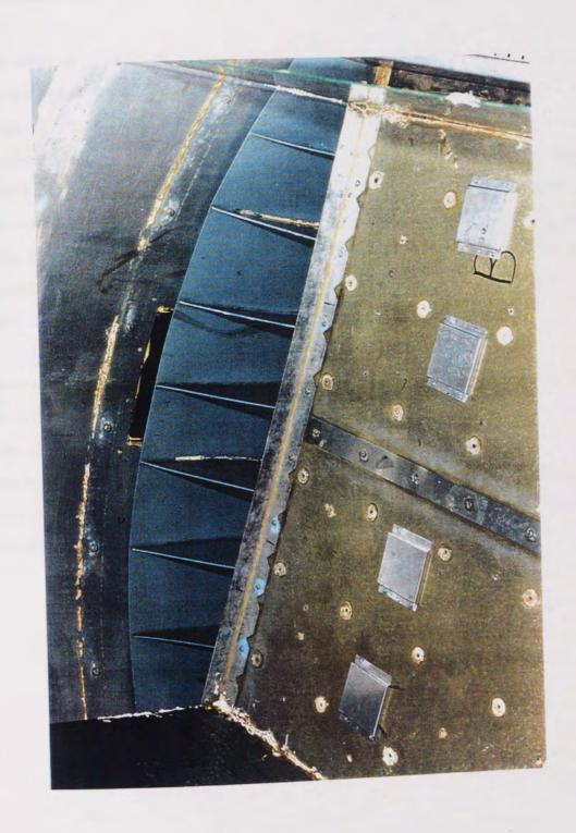
Fig. 7.7 Photograph of slotted rectangular sieve tray
