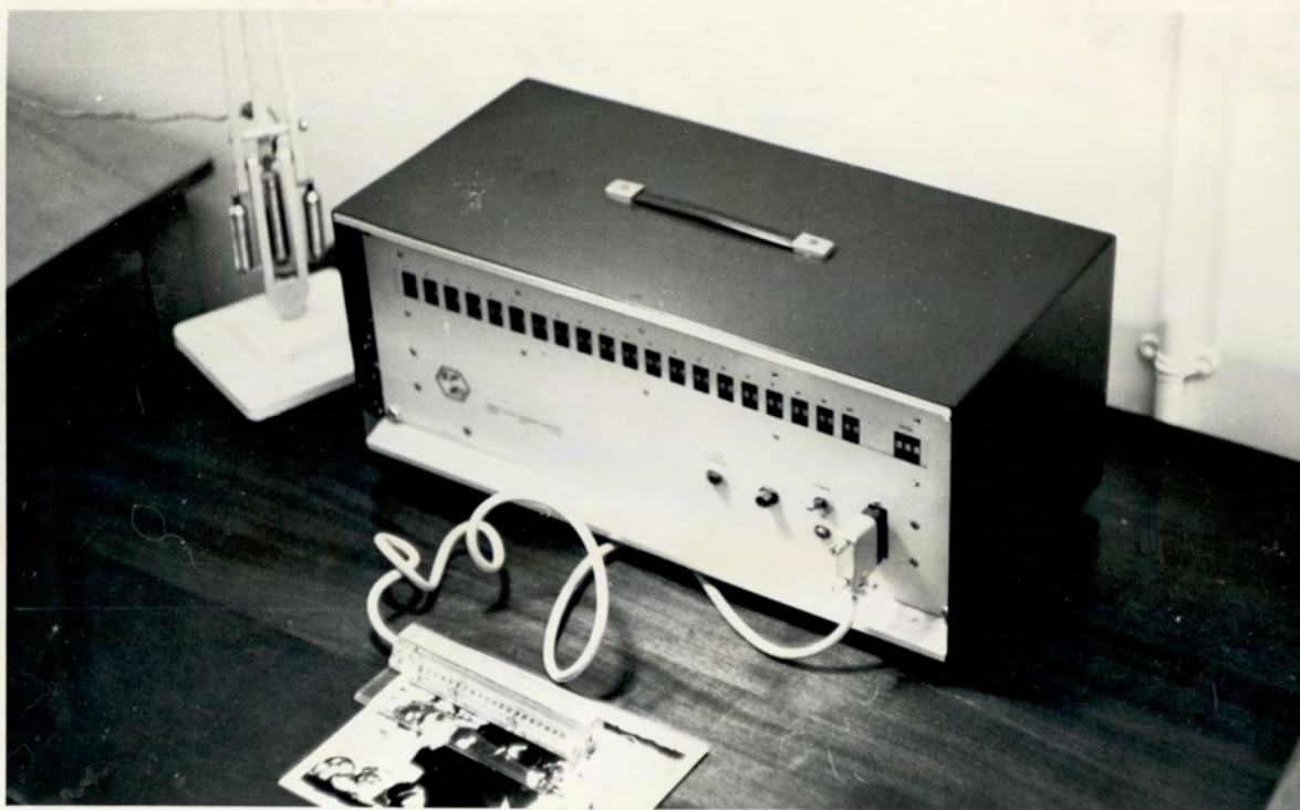
FIGURE 96. S.P.R.I. PARTICLE SIZE ANALYSER TYPE II. (136) in use for the determination of drop size distribution.
