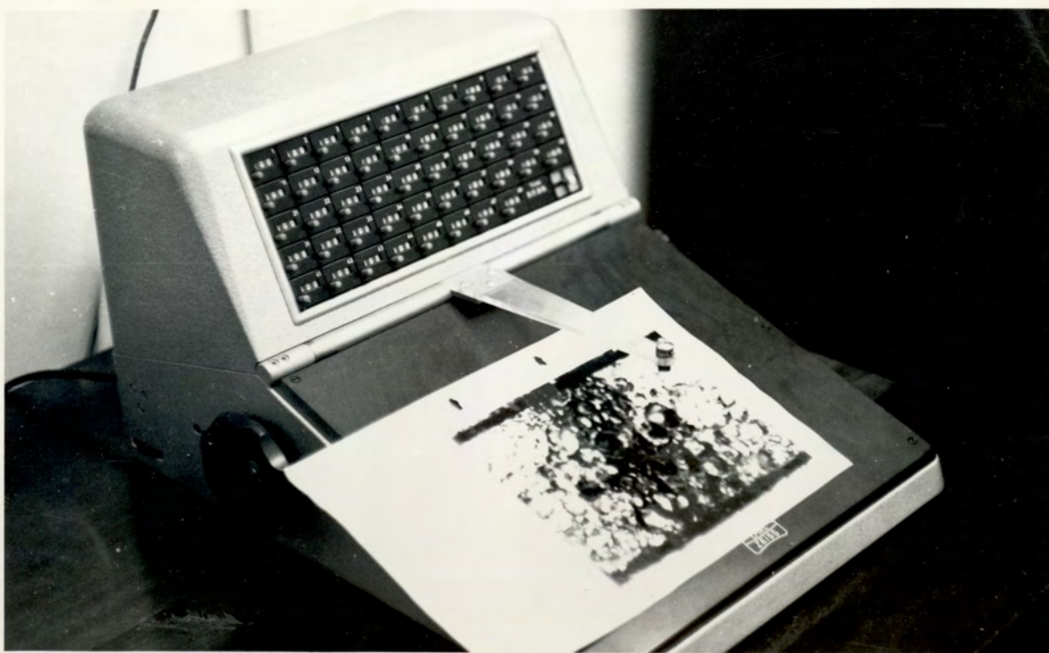
FIGURE 97. ZEISS ANALYSER T.G.2.3. (137) in use for the determination of drop size distribution.
