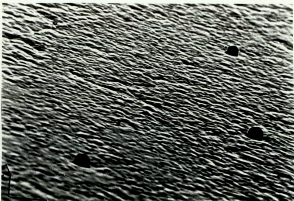
Figure 4.14 : Gold microspheres on an evaporated gold surface
