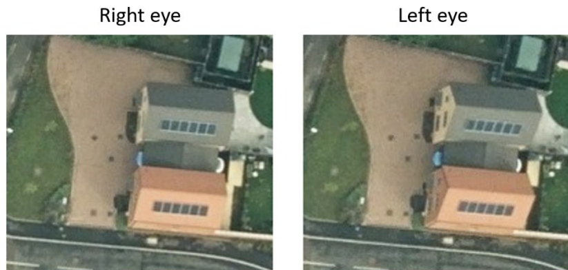
Figure 1.1: Stereoscopic pair of two houses. Binocular fusion is achievable by crossing the eyes so that the left-hand and right-hand image is seen by the right eye and left eye, respectively. © Crown copyright and database rights 2023 OS, used with permission.
