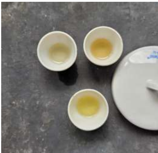
Figure 3.9 Pyrolysis waxes in ceramic crucibles for short-term ageing test.
