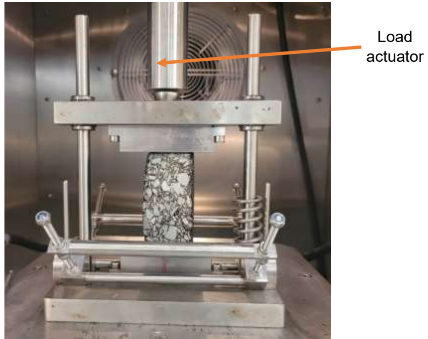
Figure 3.37 Configuration of the ITS test in the UTM-HYD machine.
