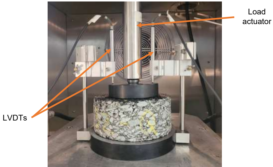
Figure 3.35 Configuration of the RLAT test in the UTM-HYD machine.
