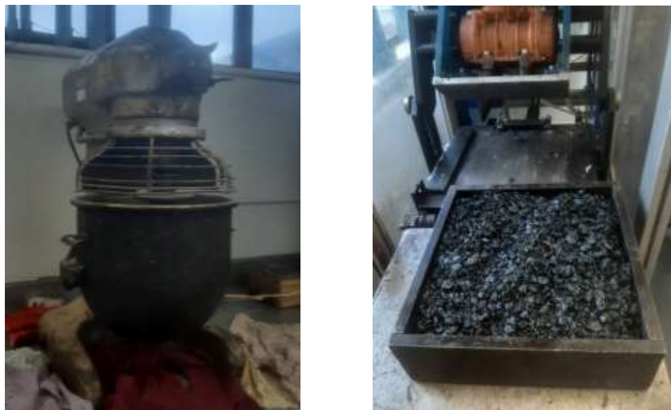
Figure 3.32 (Left) Mechanical asphalt mixer; (Right) Laboratory Roller Compactor.
