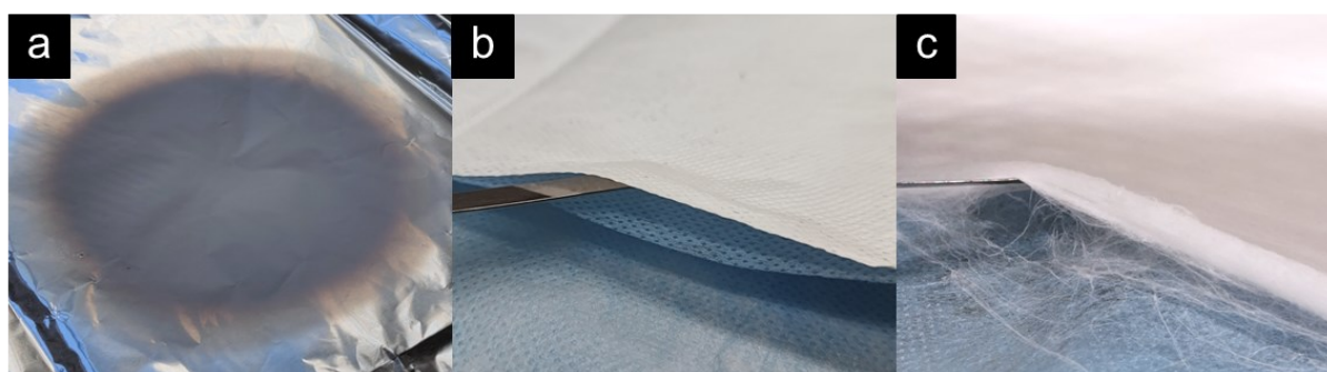
Figure 2.17. Photographs of PVA electrospun onto their respective substrates via (a) needle DC, (b) needleless DC, and (c) AC electrospinning.
