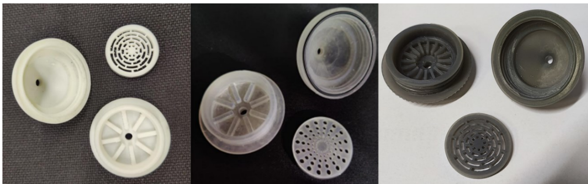
Figure 4.9. 3D printed prototypes of the third design iteration produced by SLA printing, produced using FormLabs White Resin (left hand side), Clear Resin (middle), and Tough 1500 Resin (right hand side).
