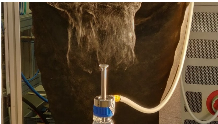
Figure 2.10. Photograph of nanofiber plume of 99% DH PVA (8% w/w concentration in water) produced by AC electrospinning.
