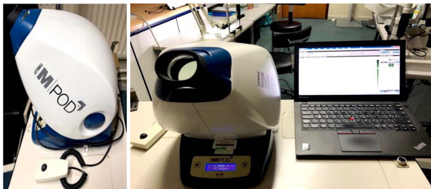
Figure 2.8: Macular pigment screener MPS9000 / MPSII, (Latif, 2019)
