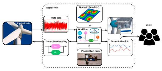
Fig. 11. Example DT for a wind farm based on [48].
