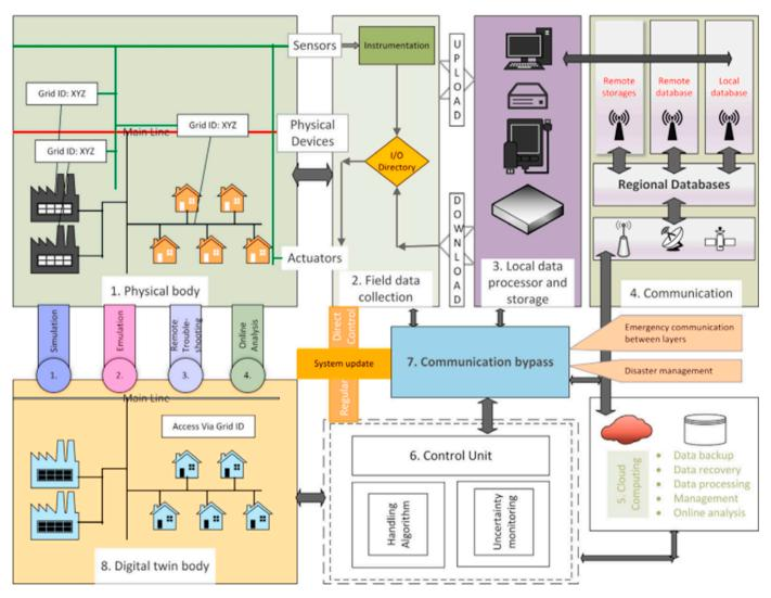
Fig. 16. Conceptual framework of electric digital twin grid [57].
