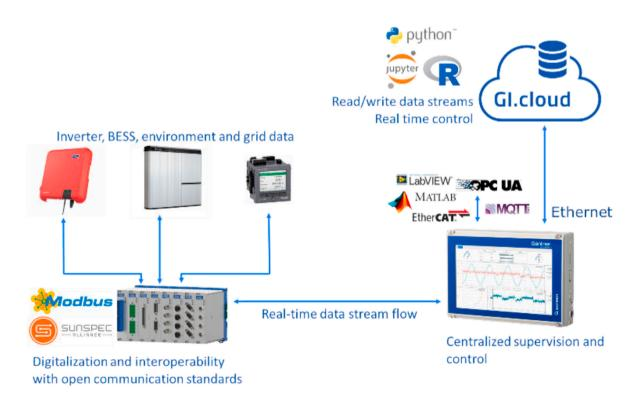
Fig. 8. Multi-service monitoring system architecture for grid-edge control and AI-driven smart grid service by Ref. [43].
