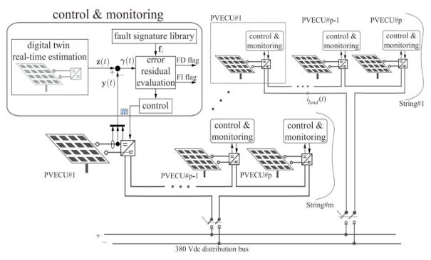
Fig. 7. Example DT Architecture in a PV system based on [40].
