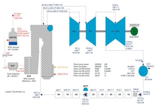
Fig. 14. Example of DT architecture for thermal power plant by Ref. [33].
