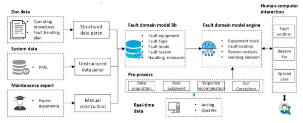
Fig. 10. Architecture of the hydropower plant fault diagnosis application [47].
