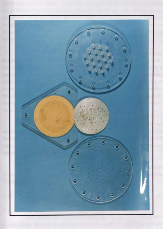
Fig. 4.5: Photograph showing the distributors used in the fluidised bed systems
