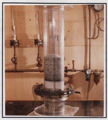
Fig.10.64: Position of the flotsam band @ Uo = 0.59 m/s
