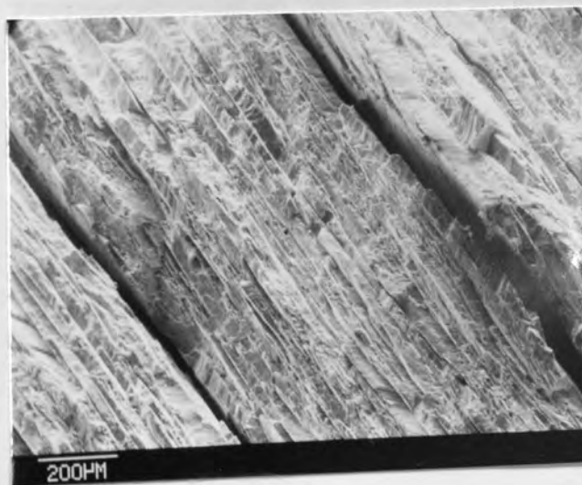
Figure 85: Fast fracture surfaces in 8090-T6 fatigue specimens.
