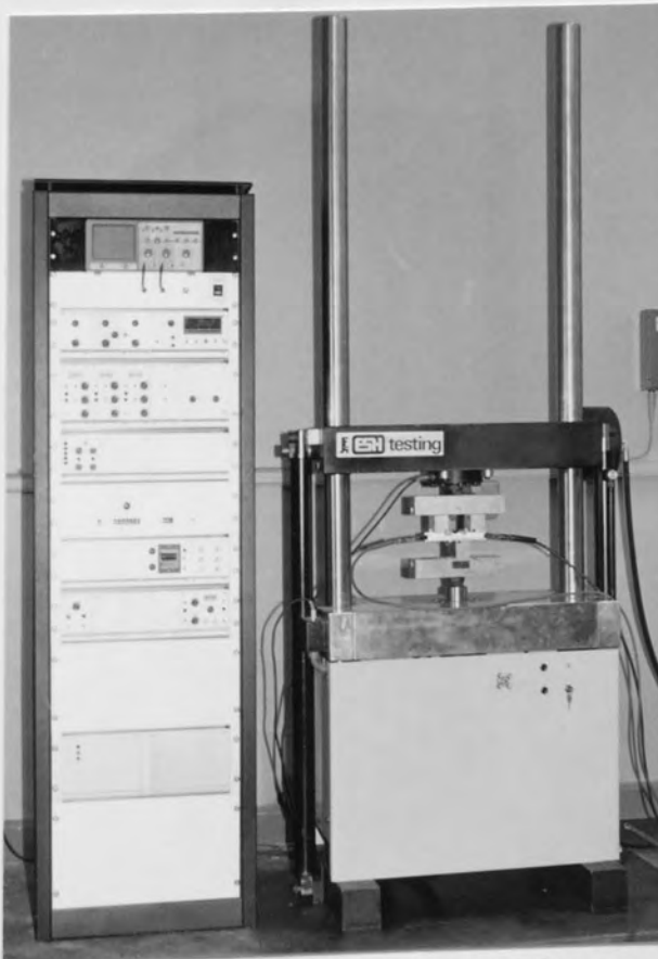
Figure 36: ESH 50kN electrohydraulic fatigue testing machine.
