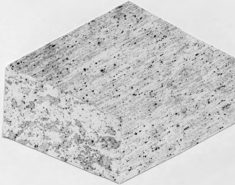
Figure 54: Grain structure of 2014-T6 (x68).
