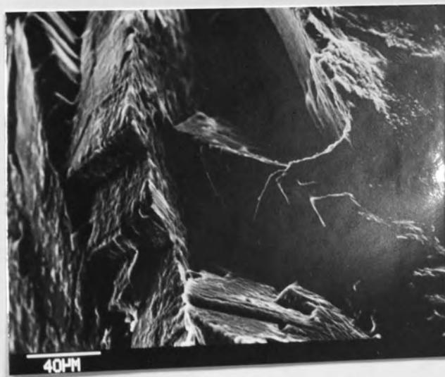
Figure 89: Corrosive attack of slip surfaces on 8090-T6 corrosion fatigue surfaces.
