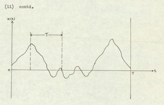
Fig. 2-2 Autocorrelation measurement.
