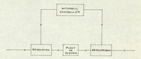
Fig.1-2. Basic arrangement of Automatic Control System.
