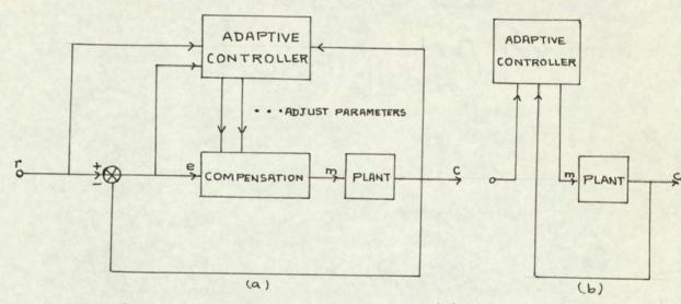
Fig. 6-5 Control-signal modification. (a) Parameter adjustment. (b) Control signal synthesis.
