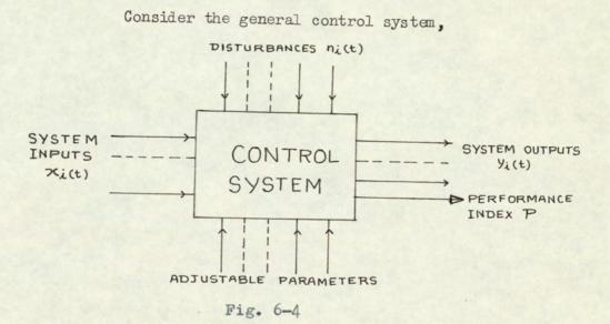
where the variables  $x_i(t)$  and  $y_i(t)$  are the normal input and output of the system. The signals  $n_i(t)$  are unknown disturbances. P is a measure of performance of the system,
