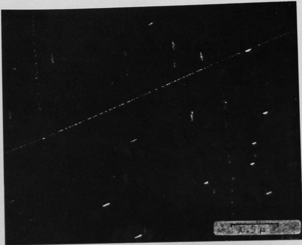
Fig.5.26 Dark field image taken with weak precipitate diffraction spot of material aged at 450°C.
