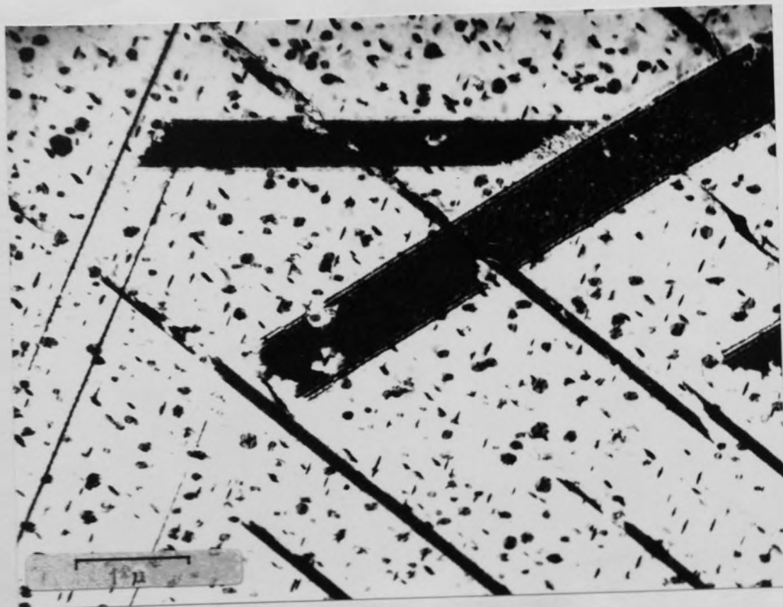
Fig.8.2 Islands of perfect crystal created within stacking faults, the smallest of which are 250\text{\AA} radius.
