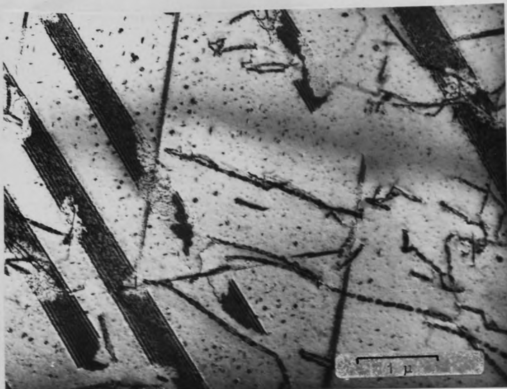
Fig.5.13 Aged at 500°C for 1 hour. .
