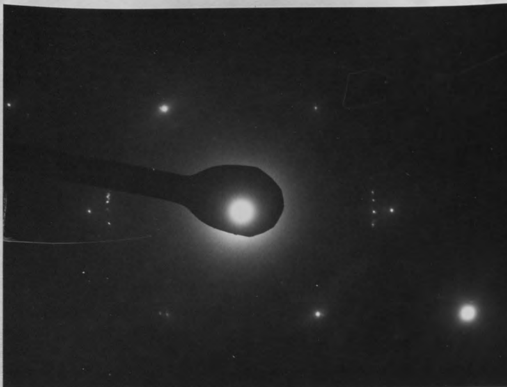
Fig.4.16 Typical selected area diffraction pattern from alloy aged at 600°C showing chromium precipitate spots superposed on the copper matrix diffraction pattern. Foil orientation near (110).
