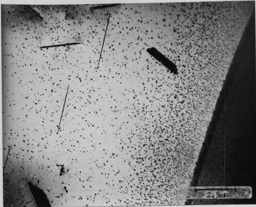
Fig.5.23 Stacking fault behaviour near grain boundary regions of precipitate enhancement.
