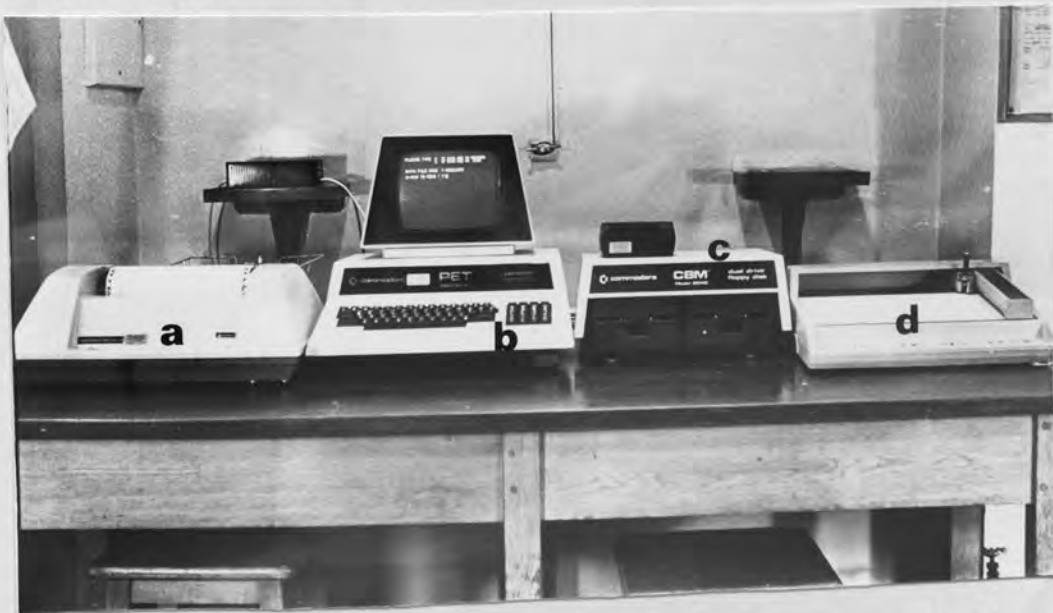
Figure 5.1: Mini-computer system used in developing field calculation, aberration and plotting programs; a) Anadex printer, b) PET mini-computer, c) c) Disk unit and d) HP plotter.
