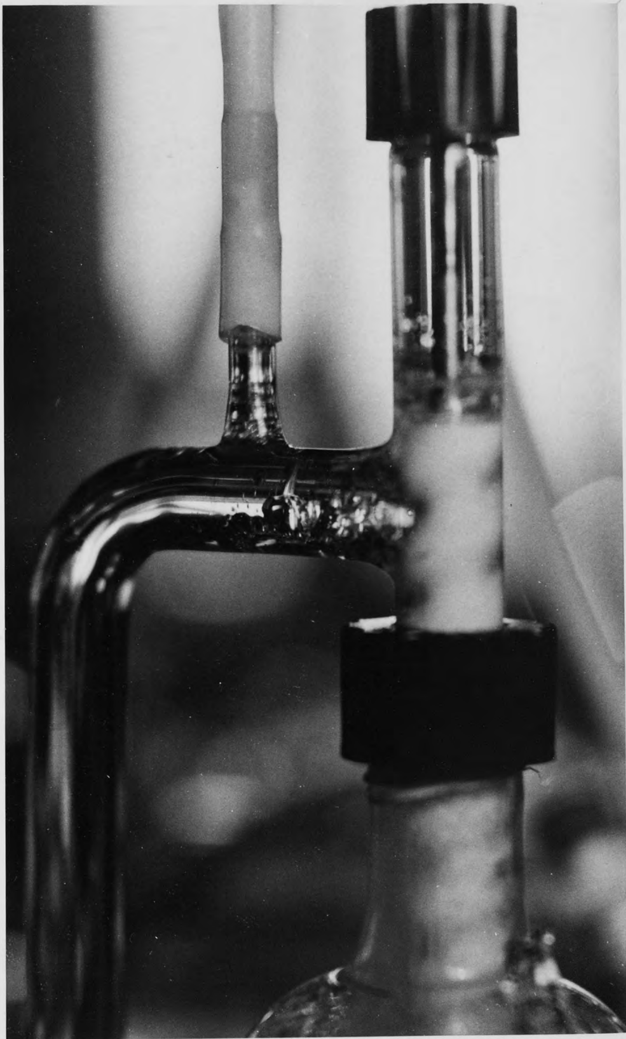
Fig .5.5 The agitator and draught tube
