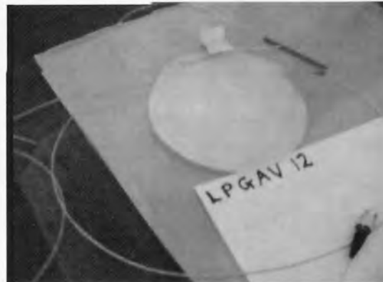
Fig. 107 Broken LPG with Helium Neon laser showing position of fracture.
