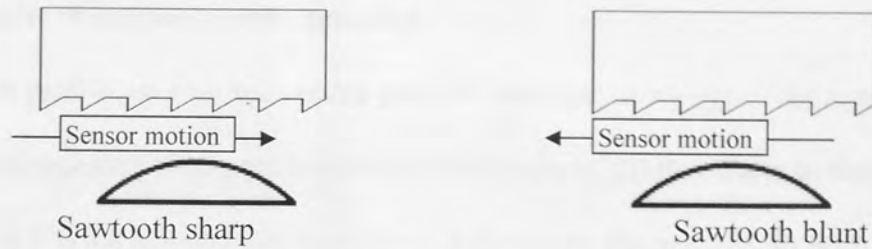
Fig 118 Sawtooth block showing 'sharp' and 'blunt' directions.
