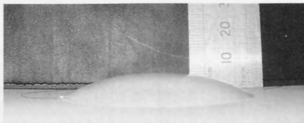
Fig. 108 Sensor with smaller encapsulation design, side view.
