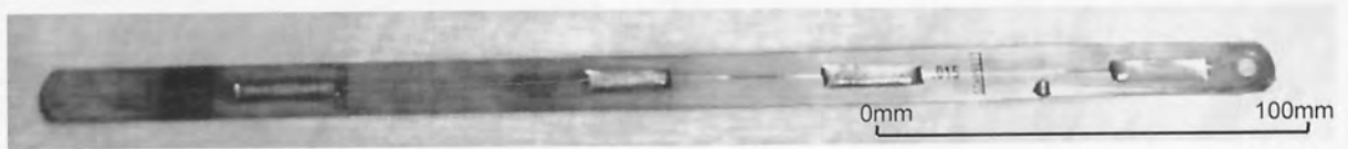
Fig. 47: Sensor layout on 1-D tactile sensing strip. (0.38mm thick)
