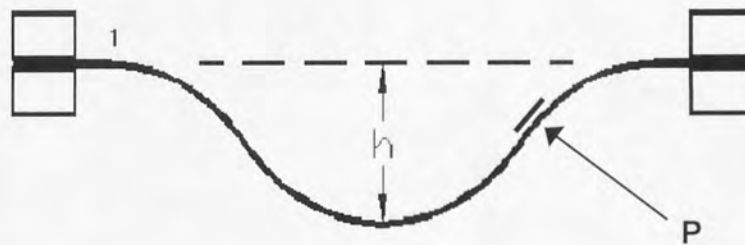
Fig. 32 Location of grating with double spectral peak on steel strip.
