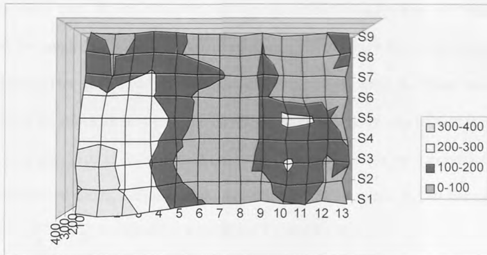
Fig.72 Plot of x errors (mm) v position, horizontal sensor arrangement
