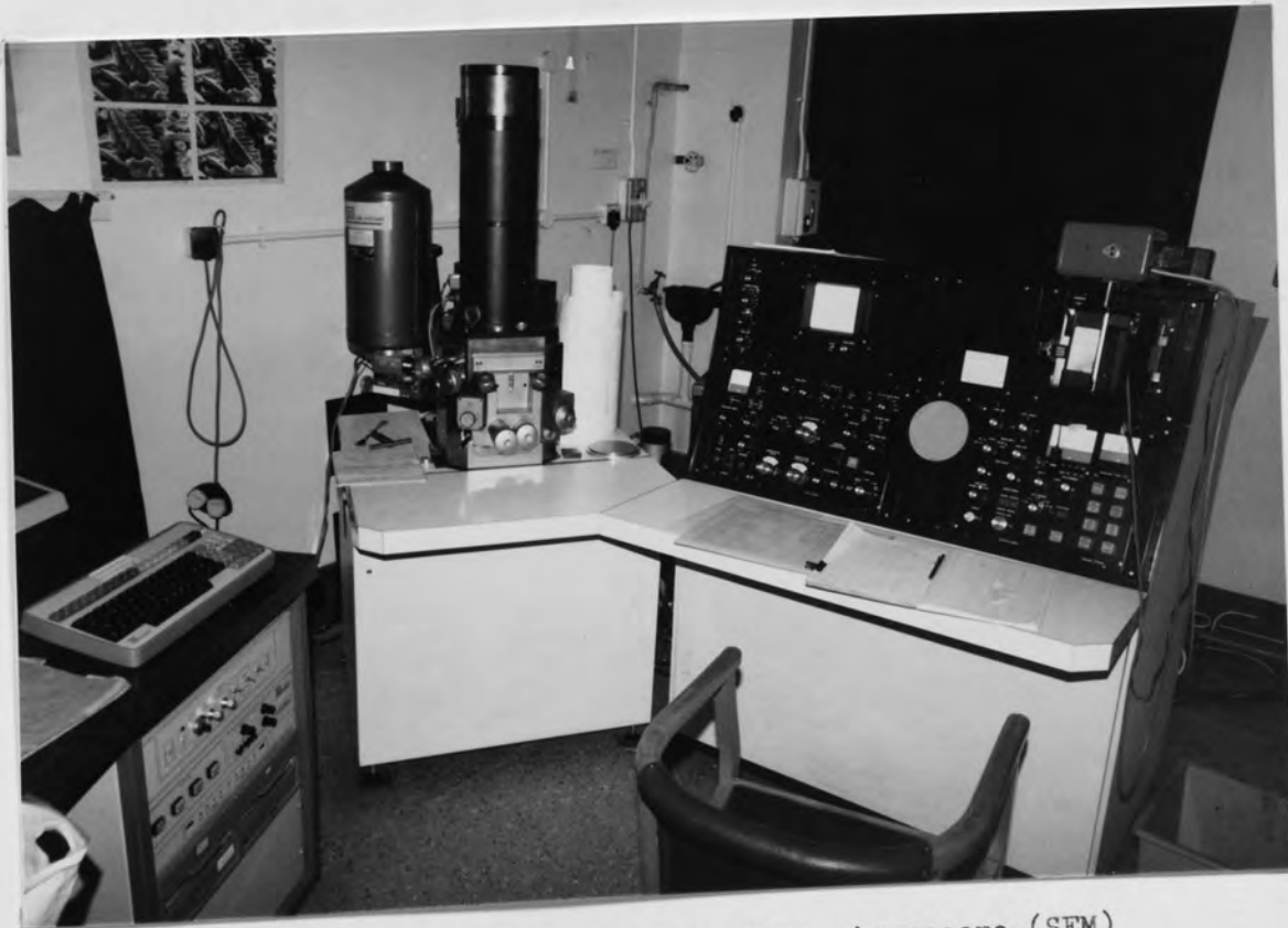
Plate 202 Cambridge S150 scanning electron microscope (SEM) with Link energy dispersive spectrometer (on left).
