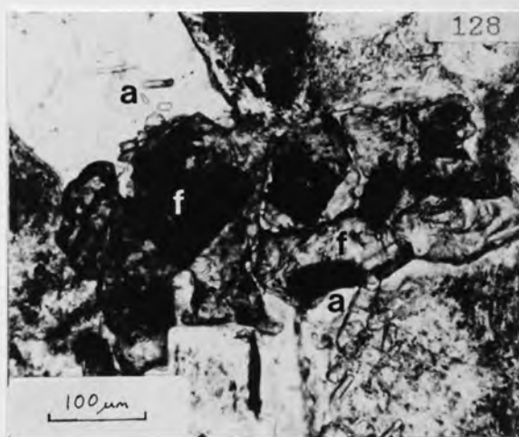
Fluorite with dark-purple cores (f). Apatite crystals (a) are included in quartz and the matrix. Arkose, BH.2, 1.9m.
