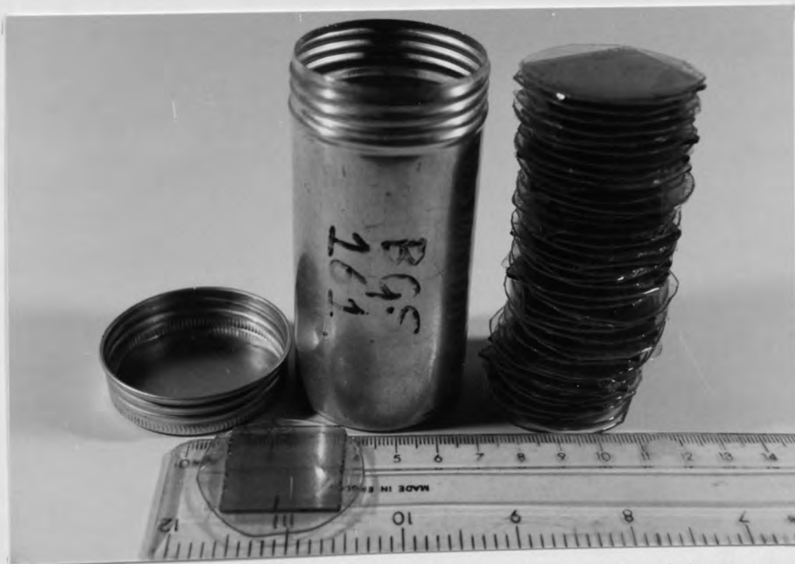
Plate 199 Circular Lexan fission track detectors attached to square polished sections. 40 sections are stacked inside the aluminium container, such that Lexan overlays are in direct contact, back to back for each pair of sections.
