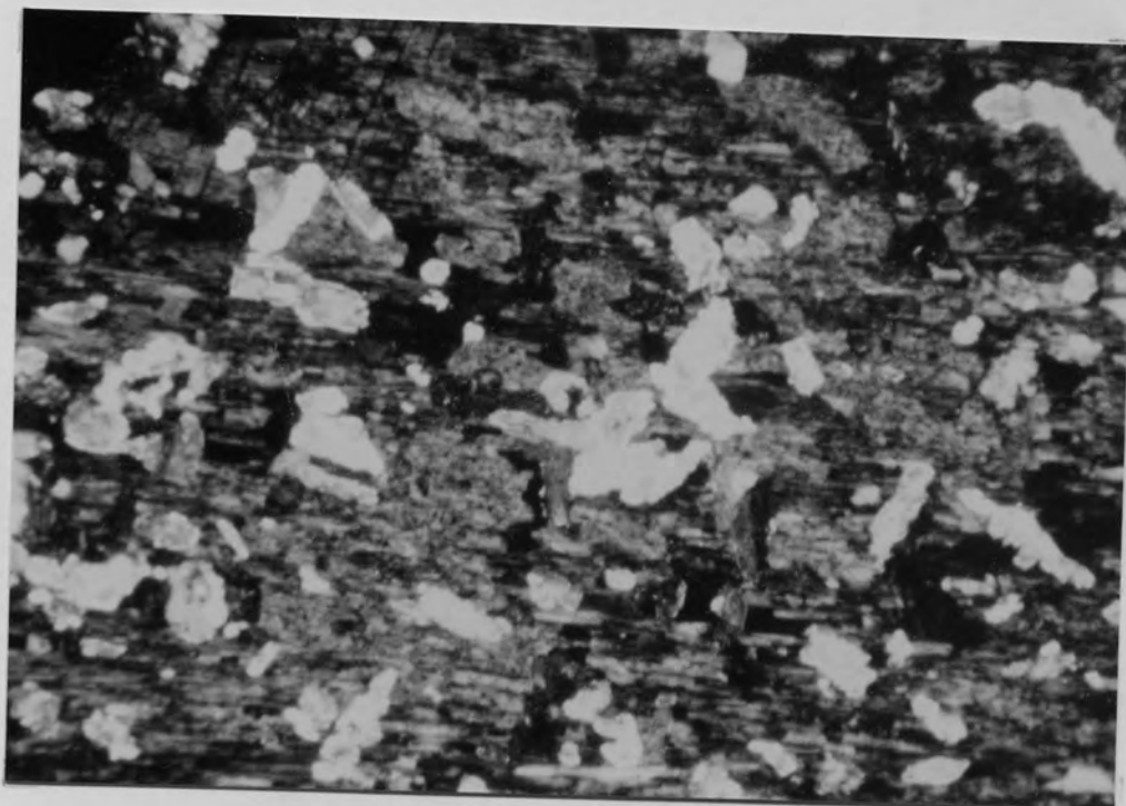
Plate 22 White mica replacing microcline in the greisenised granite (125 m).
