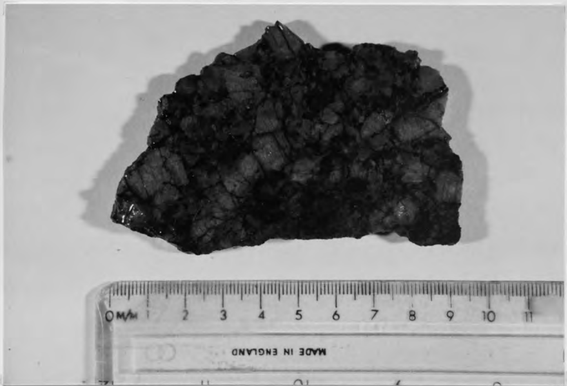
Plate 125 Reddened, porphyritic granite from Allt na Muic (Location 12)
