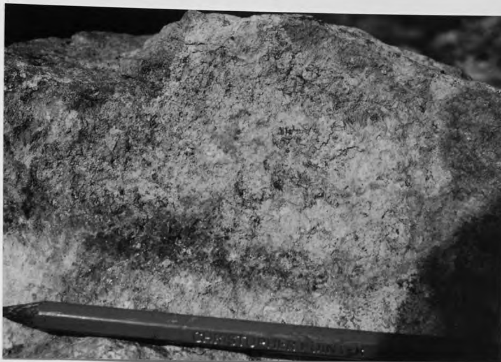
Plate 134 Joint coatings of secondary uranyl minerals in Ousdale arkose from Anomaly 5.
