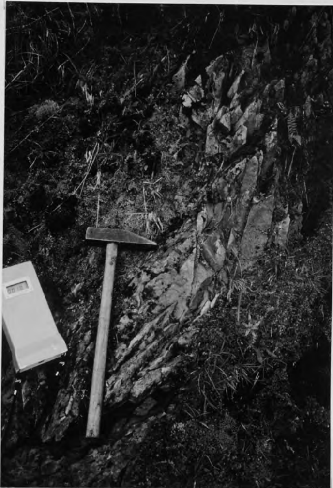
Plate 124 Fractured and reddened, radioactive granite, giving 181 cps. Location 42, Caen Burn.
