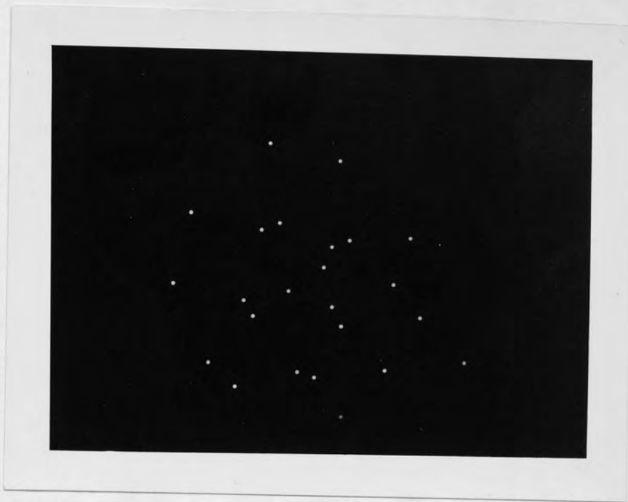
Figure 3.22 Crosscorrelation pattern of two similar 5 random-dots transparencies, one rotated by 90^\circ with respect to the other
