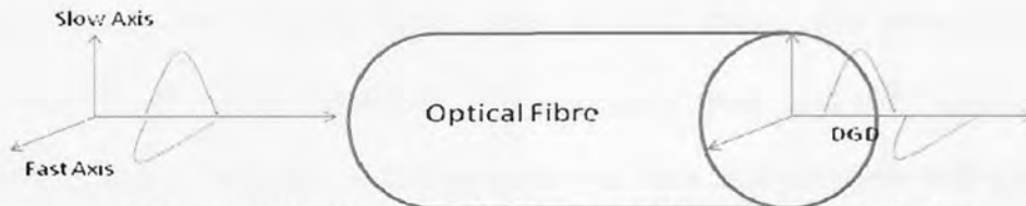
Figure 1.12: Graphical Depiction of Polarization Mode Dispersion
