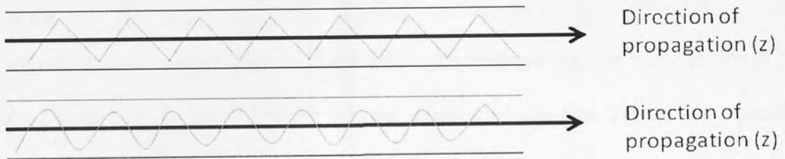
Figure 1.5: Propagation profile of the refractive index of a) Step-Index fibre and b) Graded-Index fibre.
