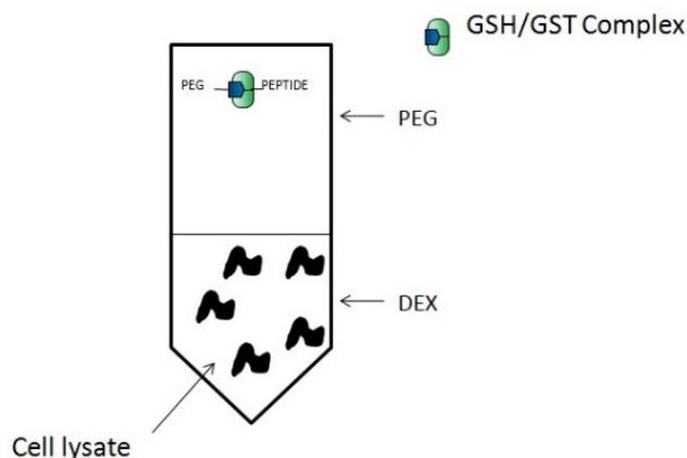
**Figure 4.1: Schematic of an ATPS system comprising a lower DEX phase and upper PEG phase.** Cell lysate containing the GST-GFPuv fusion protein was added to the system along with PEGylated GSH.
