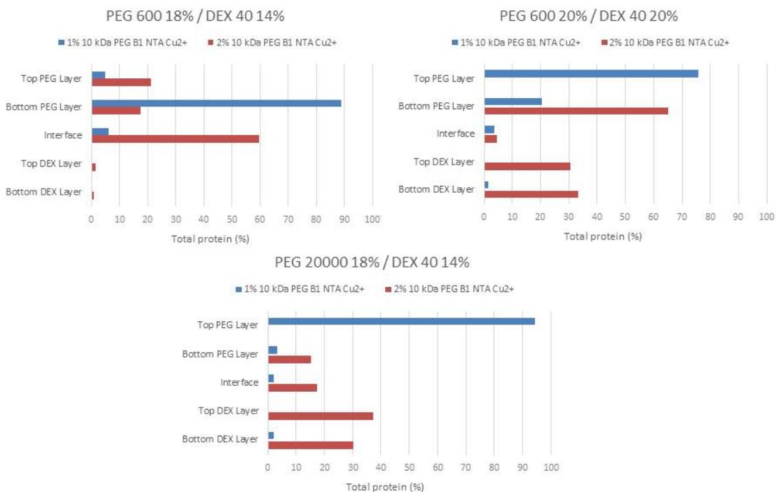
**Figure 5.6: Total protein partitioning in ATPS, composed as labelled supplemented with 1% 10 kDa PEG B1 NTA Cu<sup>2+</sup> or 2% 10 kDa PEG B1 NTA Cu<sup>2+</sup>. ATPS were set up as described in methods (2.8.16) using 100 µl of crude cell lysate expressing his-tagged GFPuv as a test sample.**
