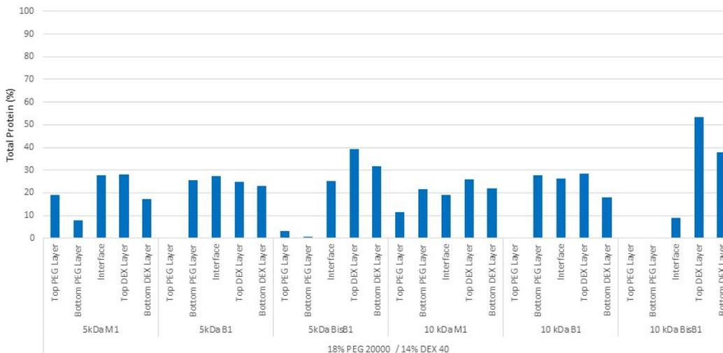
**Figure 5.9. Protein partitioning of Total Protein in ATPS composed of 18% PEG 20000 / 14% DEX 40 with 2% of overall PEG being functionalised (PEG-NTA-Cu<sup>2+</sup>) as described. 5 µl samples were taken from both the top and bottom of the PEG and DEX phases along with a sample from the interface. These were analysed using the microplate Bradford assay as described in method 2.8.15.**
