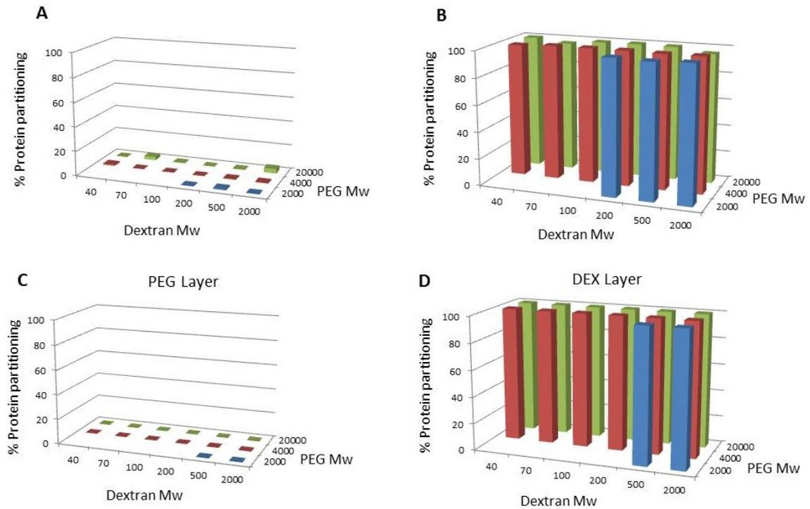
**Figure 3.3: Phase partitioning of cellular protein to upper PEG (A) and lower DEX (B) phases when utilising the settling methodology.** The phase partitioning to upper PEG (C) and lower DEX (D) phases of centrifuged systems are also shown (2000g for 2 minutes).
