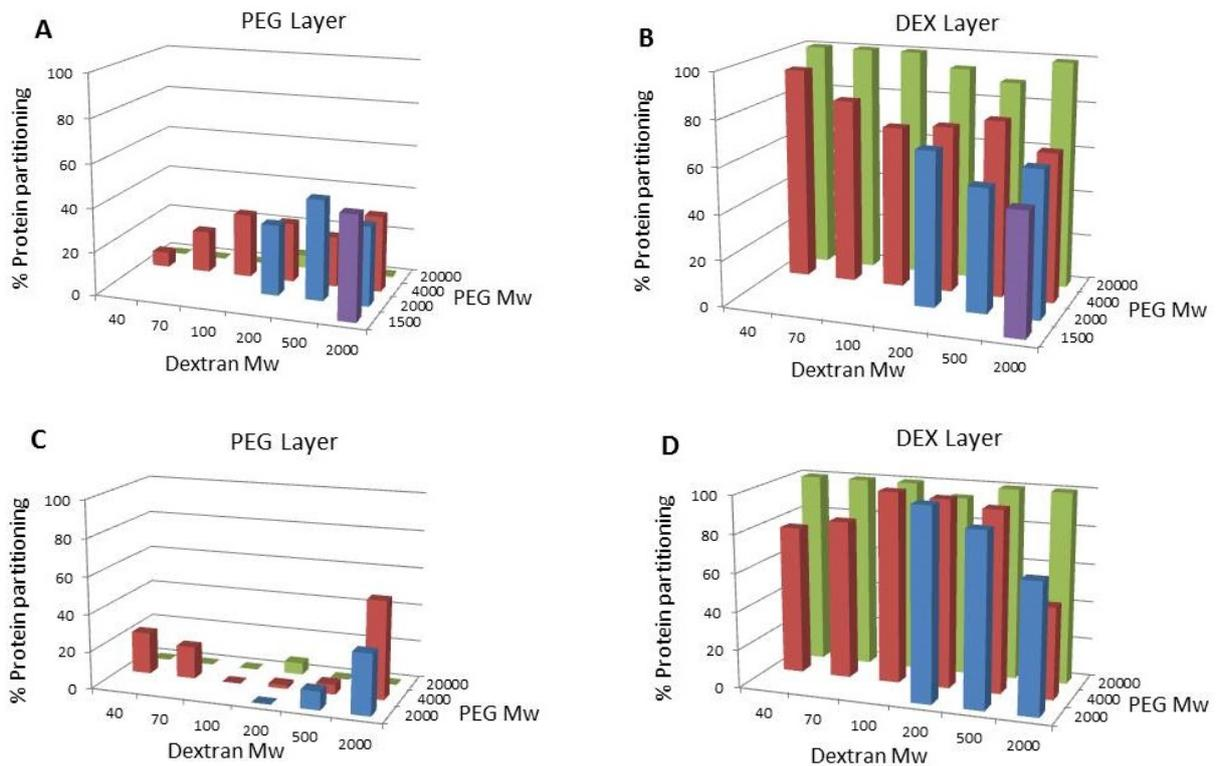
**Figure 3.5: Phase partitioning of 100µl purified GFPuv to upper PEG (A) and lower DEX (B) phases when utilising the settling methodology.** The phase partitioning to upper PEG (C) and lower DEX (D) phases of centrifuged systems are also shown (2000g for 2 minutes).
