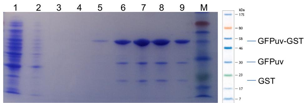
**Figure 4.3: Polyacrylamide gel electrophoresis of GST-GFPuv purification.** 12% PAGE gel, stained with Coomassie Blue. Lanes: 1) Column flow through; 2-4) Washes 1-3; 5-9) Elutions 1-5; M) 15  $\mu$ l NEB ColorPlus™ Prestained Protein Marker, Broad Range (7-175 kDa). All other samples were 5  $\mu$ l of original material.
