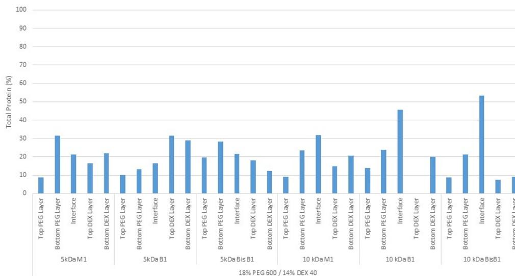
**Figure 5.7. Protein partitioning of Total Protein in ATPS composed of 18% PEG 600 / 14% DEX 40 with 2% of overall PEG being functionalised (PEG-NTA-Cu<sup>2+</sup>) as described. 5 µl samples were taken from both the top and bottom of the PEG and DEX phases along with a sample from the interface. These were analysed using the microplate Bradford assay as described in method 2.8.15.**
