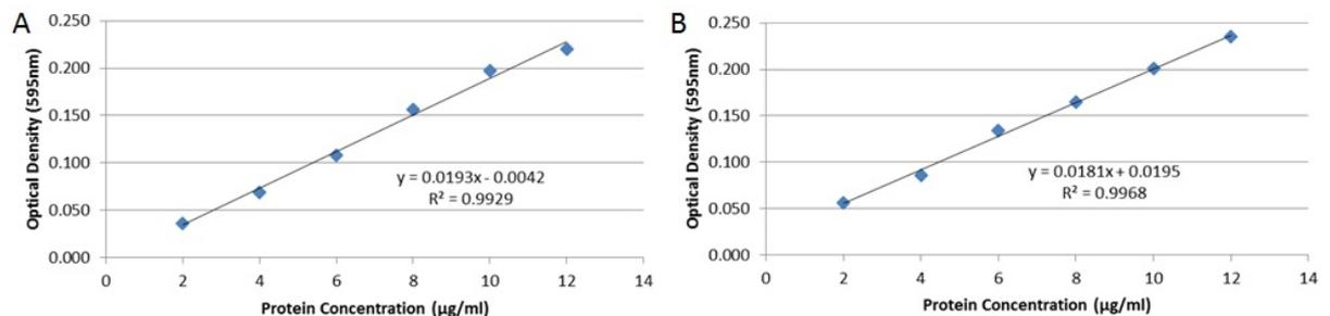
**Figure 3.2: Bradford assay standard curve for settled (A) and centrifuged (B) systems.** The standard was produced using known concentrations of BSA prepared from stock solution as described in section (2.2.8) of “Materials and Methods”
