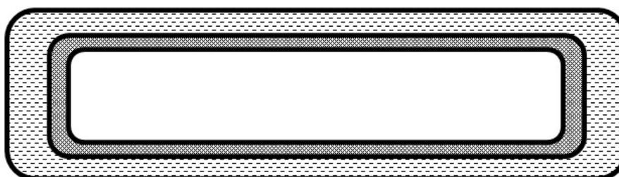
Figure 3.14 Schematic of a bilayer coating (shaded regions) around a tablet core
