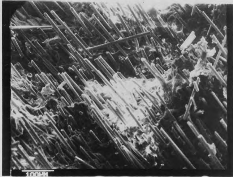
Plate 4.1 Scanning electron micrograph of the tensile fracture surface of 1%MA/0.2%DCP modified stabilised PP(HWM25) containing 30% glass fibre (A-1100 silane coupled)
