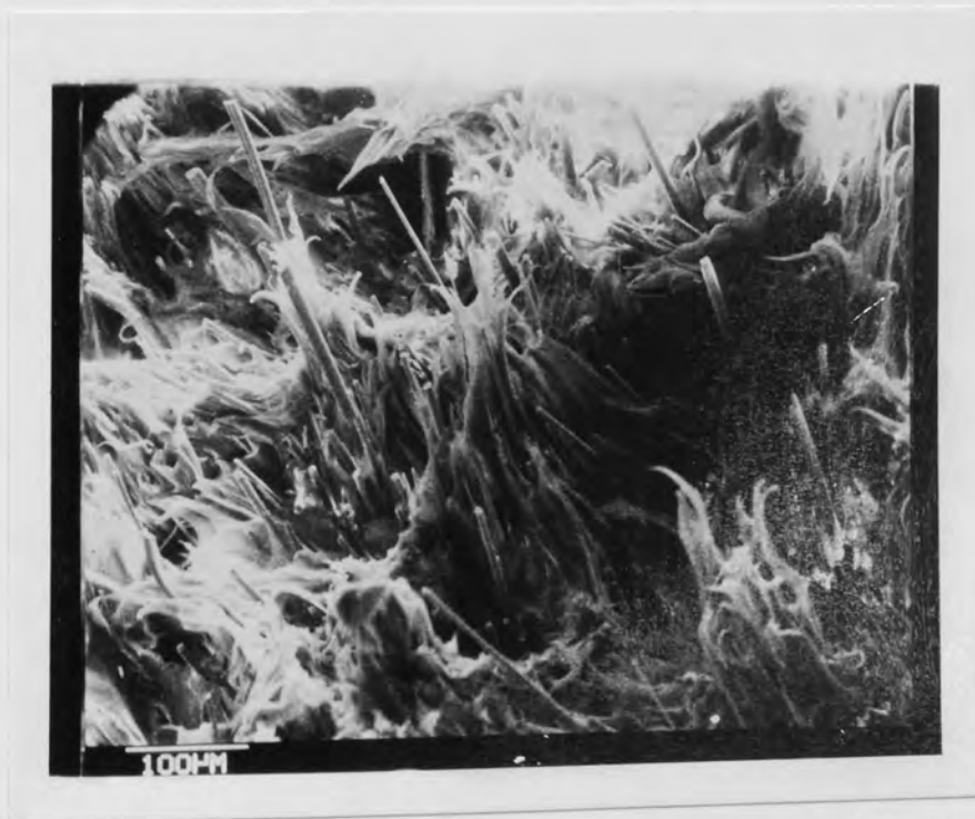
Plate 5.2 Scanning electron micrograph of the tensile fracture surface of 1%ADCT/0.2%DCP modified unstabilised PP(HF22) containing 30% glass fibre (A-1100 silane coupled) after 4 weeks Gunk immersion (65°C) 310.
