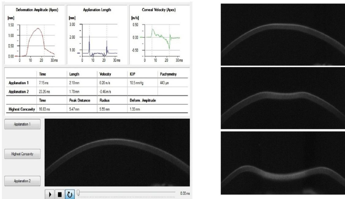
Figure 2.2 The Corvis ST (left) is able to produce detailed images of the cornea during air puff deformation. The instrument is also a validated tonometer and pachymeter.
