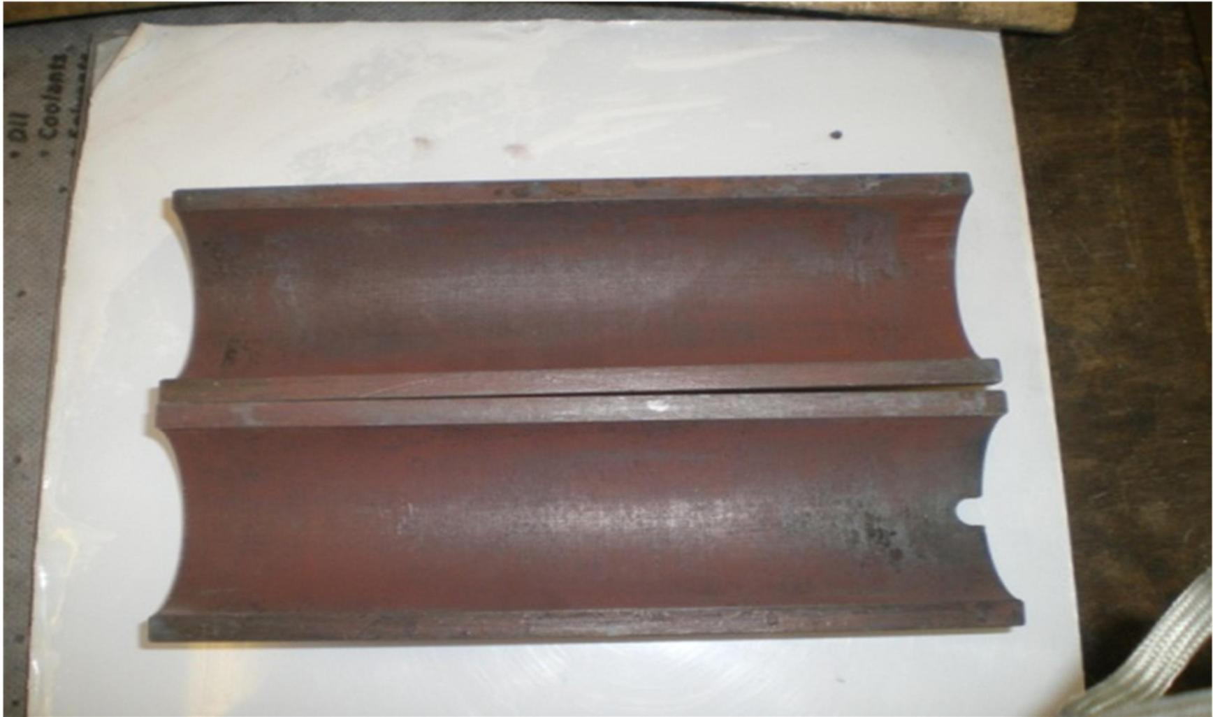
**Figure 6-23 Photograph of steel jacket after fabrication**
