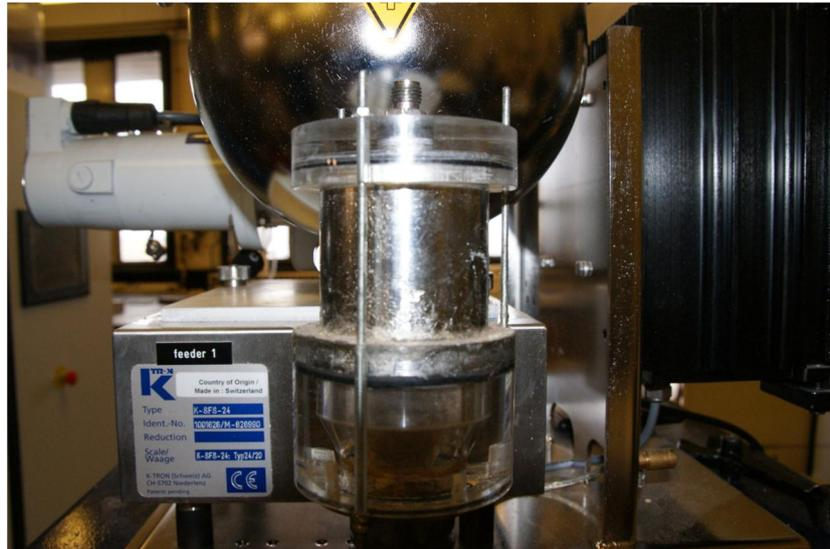
**Figure 8-6 Installed see through outlet on K-TRON KT-20 metering system**
