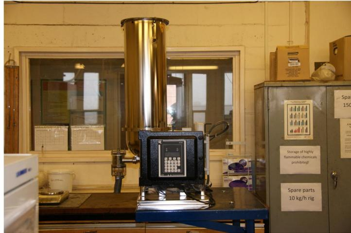
**Figure 8-4 Digital photograph of K-TRON KT 20 and mobile stand**
