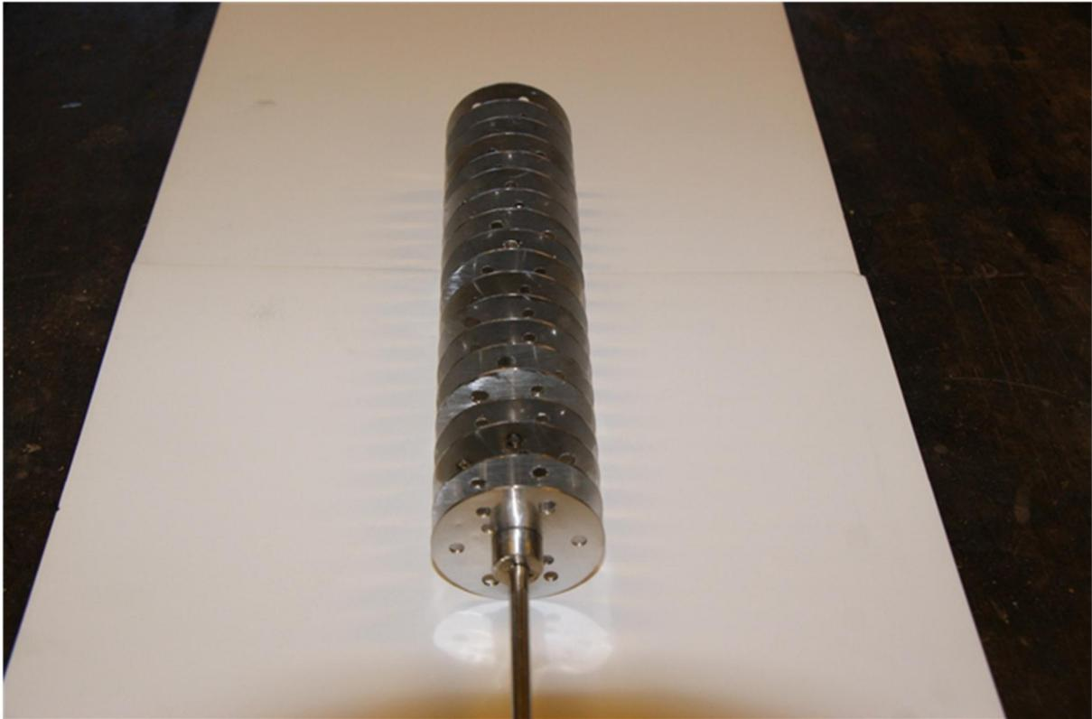
**Figure 6-10 Quench Column Plates**
