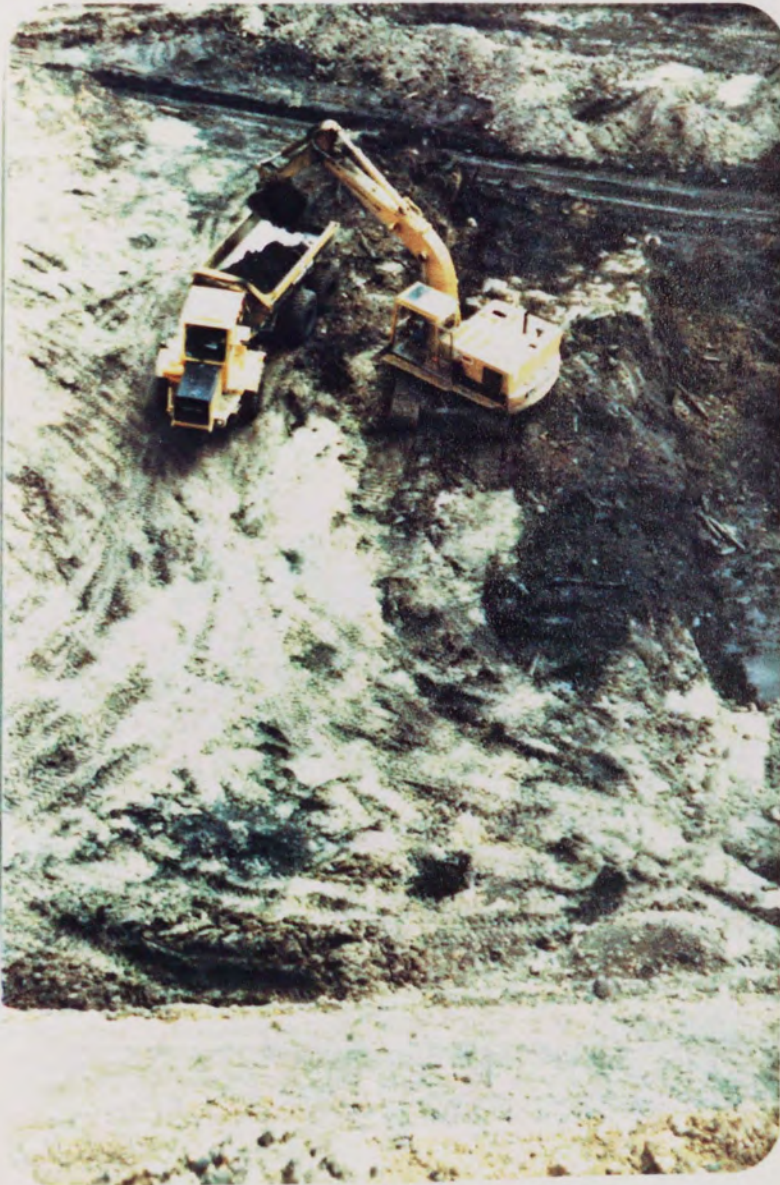
PLATE 5-3-6 Excavation of Thick Coal pickings.
