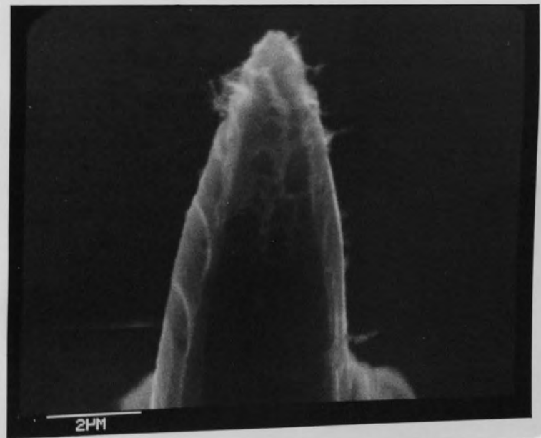
Fig. 5.12 S E M micrographs of tip profile (a) before emission, (b) after 10 mins and (c) after 1 hour of drawing emission current.
