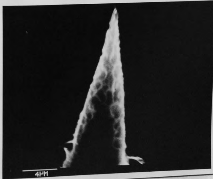
Fig. 5.2 SEM micrograph of (a) freshly etched tip (b) after outgassing extractor and (c) after drawing current.
