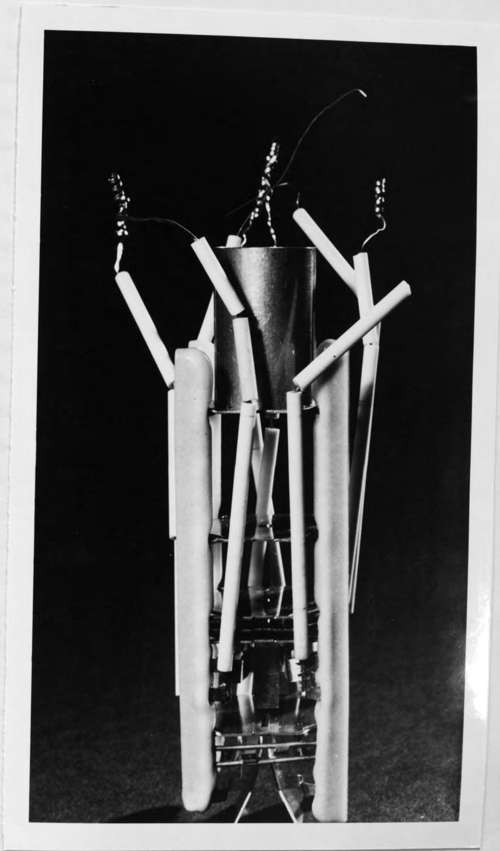
Fig. 4.48 Photograph of 300 mm focal length redesigned gun for proto type C R T.
