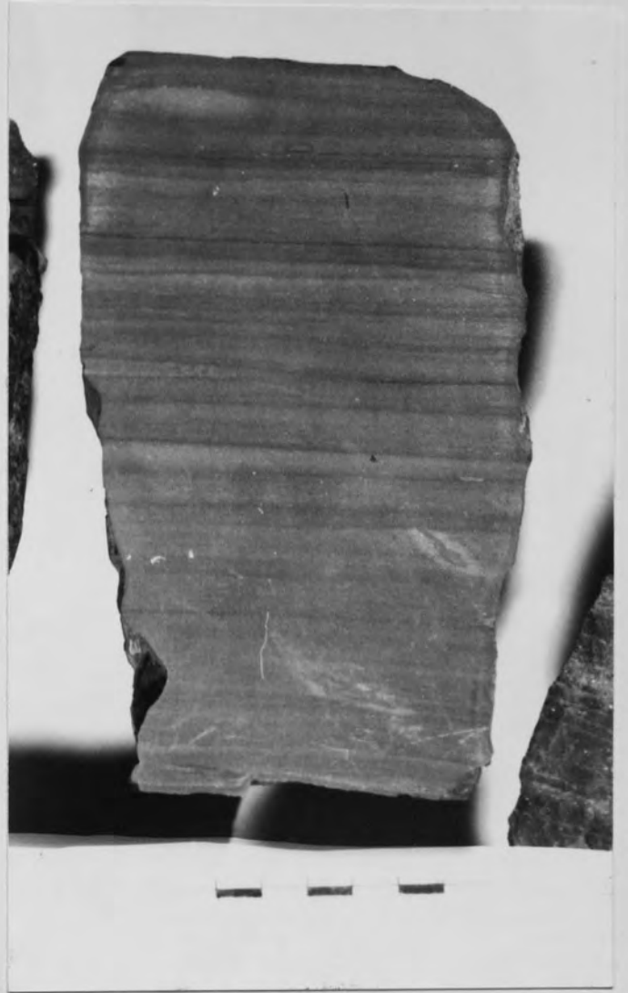
Plate 1 Typical layered blackband ironstone. Red Shagg Ironstone, Mitchell's Wood, north Staffordshire (scale bar in cm)
