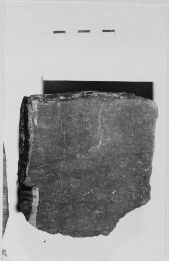
Plate 3 Blackband 'seatearth' Ironstone, Mitchell's Wood, north Staffordshire. Sample from immediate floor of thin top leaf of coal exhibiting well developed seatearth texture (scale bar in cm)
