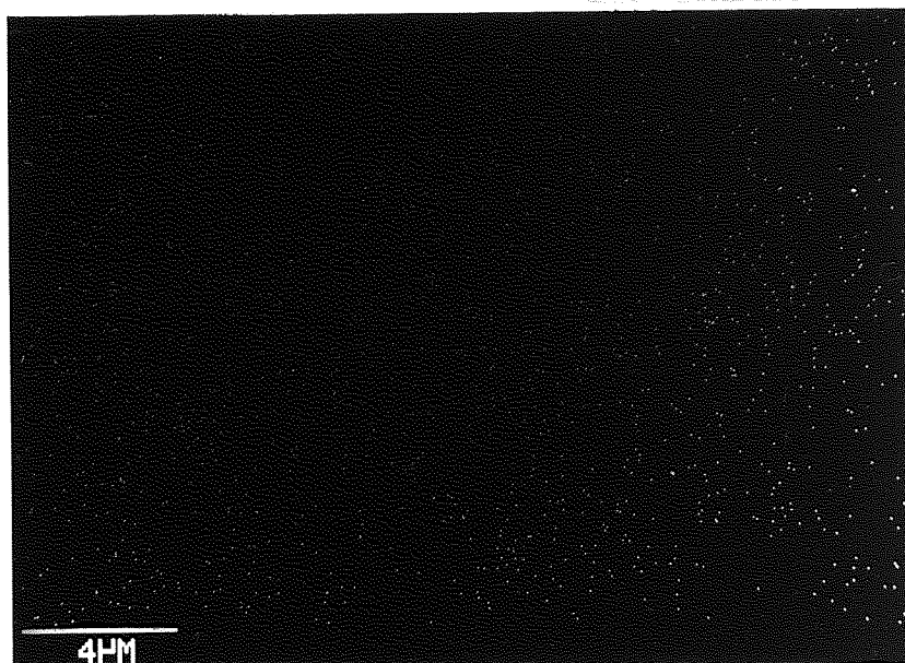
PLATE 4.6. Silicon X-ray map of the area shown in plate 4.4. (Unetched, magnification as shown) (Specimen No. P46C)
