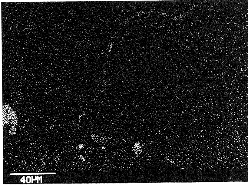
PLATE 5.13: Silicon X-ray map of the area shown in plate 5.12. Note the presence of silicon compounds in the defect (Etched in 1% Nital, magnification as marked) (Specimen No. P40C)
