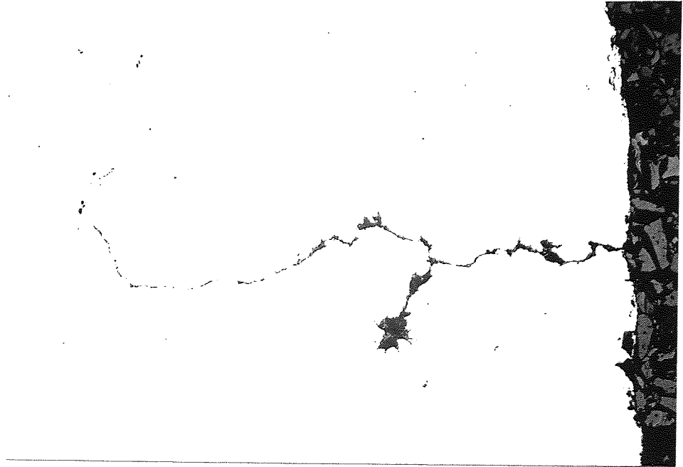
PLATE 3.2. Section through defect shown in plate 3.1. The metal surface is at the right hand edge. (Unetched, X 60) (Specimen No. P3C )
