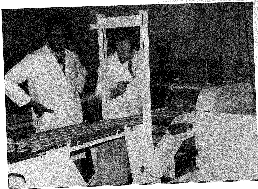
Plate 5.12 Rotary moulding of plantain biscuit at Flour Milling and Baking Research Association (FMBRA), Chorleywood.
