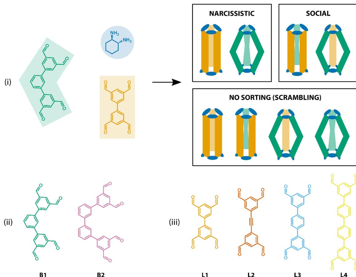
**Figure 1** (i) Illustration of narcissistically and socially self-sorted systems as opposed to non-sorted scrambled outcomes for an imine-based organic cage forming reaction using linear (green) and bent (orange) aldehydes in presence of (1*R*,2*R*)-*trans*-1,2-cyclohexanediamine (blue); (ii) structures of the bent (**B1**, **B2**) and (iii) linear (**L1–4**) tetraaldehydes used in this work.
