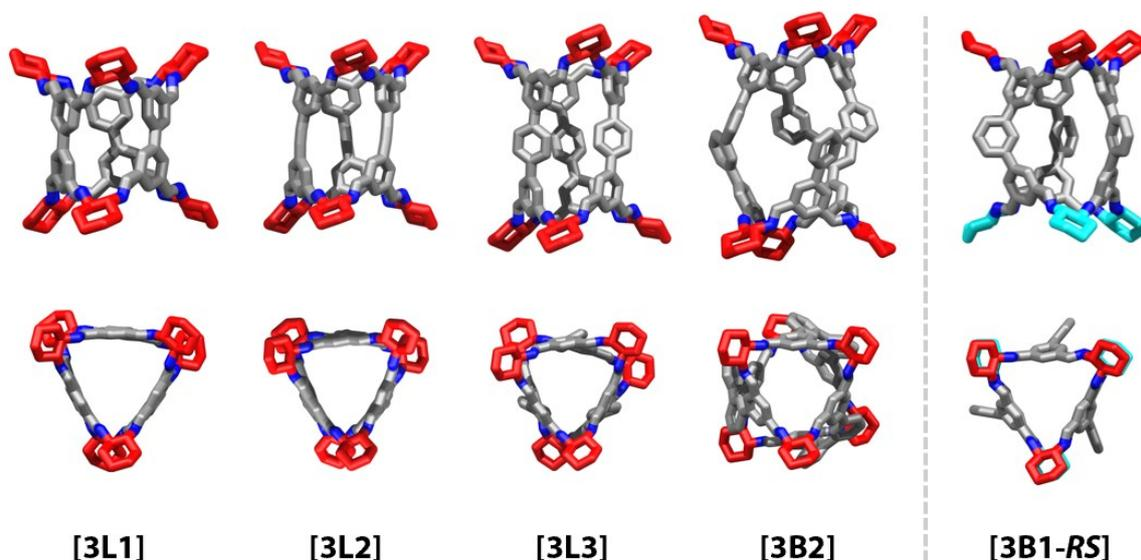
**Figure 2** Side- and top-views of the solvated single crystal X-ray structures of the imine-based cages originating from the reactions of tetraaldehydes **L1–3** and **B2** (grey) with *R,R*-CHDA (red). For **B1**, single crystals were only obtained for a pseudo-*C*<sub>3h</sub>-symmetric structure incorporating both *R,R*- and *S,S*-CHDA (cyan). Hydrogen atoms and solvent molecules are omitted for clarity, nitrogen atoms are in dark blue.
