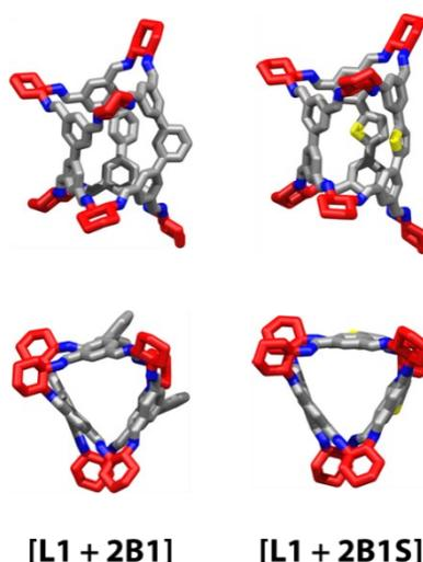
**Figure 4** Side- and top-views of the single crystal X-ray structures of the socially-sorted **[L1 + 2B1X]** cages originating from the reactions of mixtures of tetraaldehydes (grey) **L1** and **B1** (left) or **B1S** (right) with *R,R*-CHDA (red).
