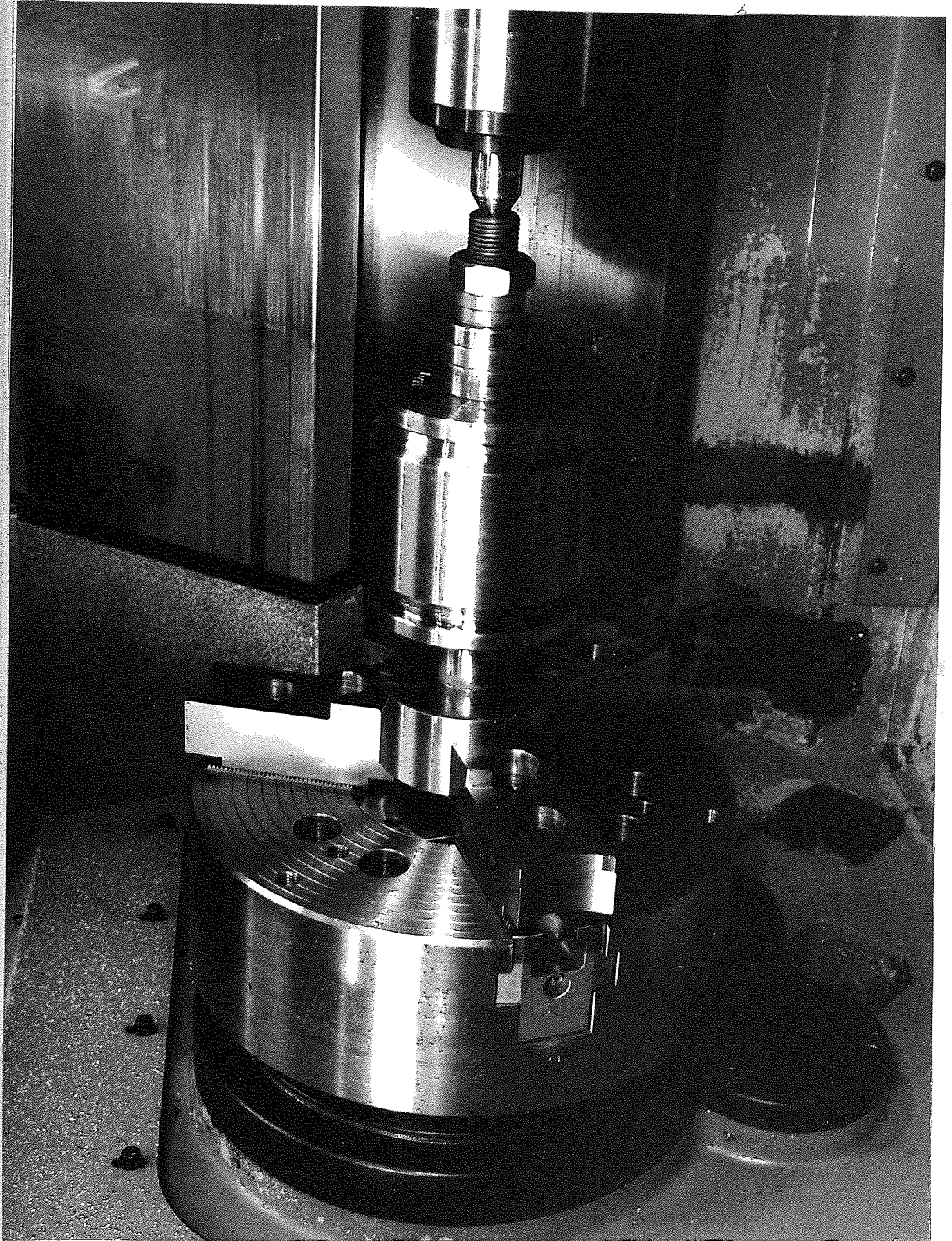
Plate 7.1 WORKPIECE SETUP USING A MANDREL
