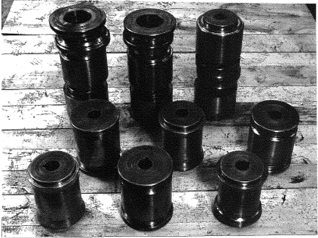
Plate 8.3 A SET OF FORM-ROLLS PRODUCED BY CNC
